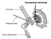
The toothed axle washer is not necessary for a quick release type
