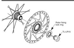
Tightening torque: 40 - 50 N·m {350 - 435 in. lbs.}
