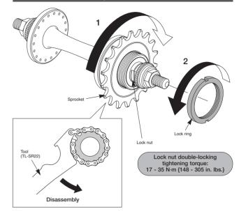
After removing the lock ring, use the TL-SR22 to remove the sprocket from the hub as shown in the illustration
