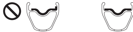
* Pull the tape with your hand to some extent when affixing it. * Do not use a tool (use your hand). Otherwise, the tape may become torn.
