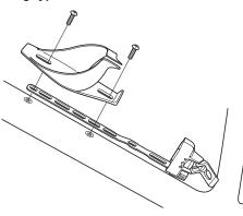
For the long type, secure it with the bolts supplied with the frame or the bottle cage.
