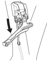
Electric wire for battery mount [In the case of a built-in battery (SM-BTR2/BT-DN110/BT-DN110-A)]
