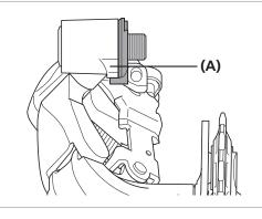
Hook the stopper plate on the stopper claw on the bracket body.
