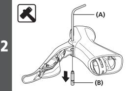
Place the lever with the shifting switch left side up as shown in the illustration.
