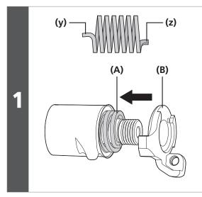
When mounting the B tension spring, insert the longer end of the spring into the bracket body side and the shorter end of the spring into the hole on the stopper plate side.
