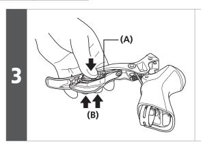
Press the switch unit by hand so that the switch springs go into the grooves in the buttons, and then push the shifting switches [X] and [Y] in as far as they will go.
