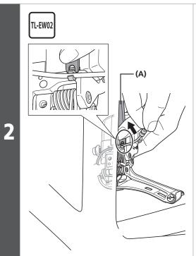
Remove the electric wire from the cable holder.
