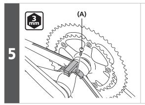
Once the electric wires have been routed, secure junction B underneath the bottom bracket shell.
