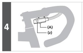
Press the button at junction A until the red LED turns off in order to switch from rear derailleur adjustment mode to gear shifting mode.
