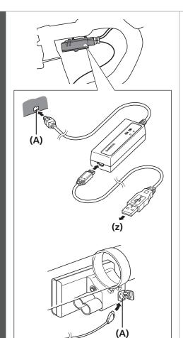
Connect the charging cable to the junction A or the charge port of the system information display.
