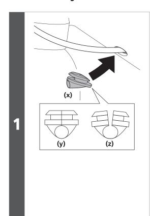
Install grommets in appropriate positions for the electric wires.
