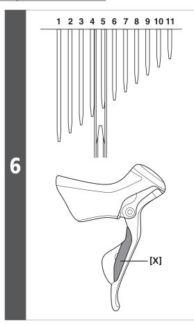
While turning the front chainwheel, operate shifting switch [X] to move the guide pulley toward the inside until the chain touches the 4th sprocket and makes a slight noise.
