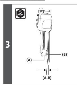
Use a 5mm hexagon wrench to secure the chain guide outer plate so that the flat part of the plate is directly above the largest chainring and so that the rear edge of the chain guide is within 0.5
