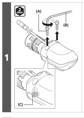
Remove two cover fixing bolts (M2.6) with a 2mm hexagon wrench.
