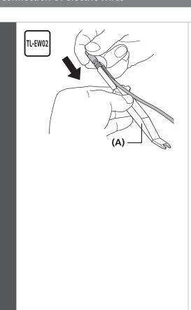
Set so that the projection on the connector is aligned with the groove on the narrow end.
