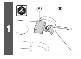
Remove the wire guide from the frame, if attached.
