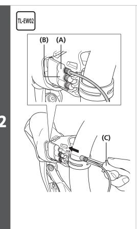
Use the TL-EW02 to connect the connector of the electric wire to the E-TUBE port on the lever side.
