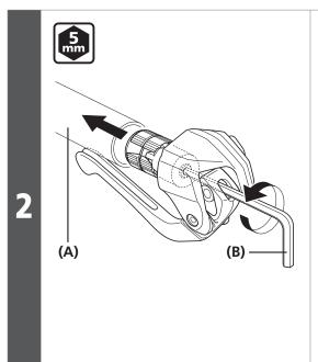
Install the brake lever to the handlebar by tightening counterclockwise with a hexagon wrench.
