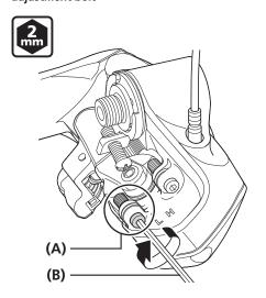
Shift the rear derailleur to the largest sprocket, and then tighten the low-side stopper adjustment bolt until it just touches the left link.
