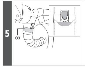
Wind on the handlebar tape.
