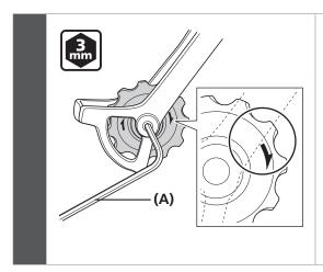
Replace pulleys using a 3mm hexagon wrench.
