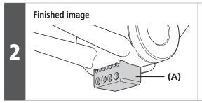
Attach junction B using the wire guide mounting hole.
