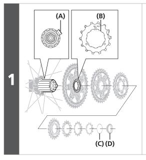
Place each sprocket with the marked side facing outward.
