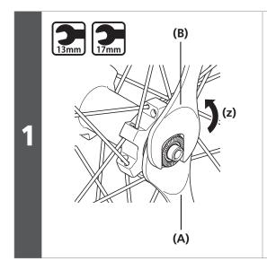
Use the hub spanners to loosen the lock nut on the double-lock section.
