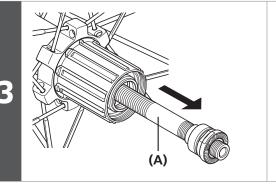
Pull out the hub axle from the freewheel body.
