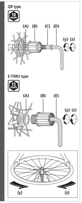
After removing the hub, remove the freewheel body fixing bolt (inside the freewheel body), and then replace the freewheel body.
