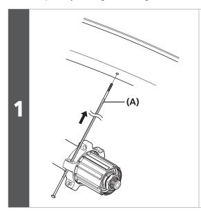
Pass the spokes through the hole in the hub flange and the hole in the rim.
