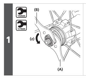
Use the hub spanners to loosen the lock nut on the double-lock section.
