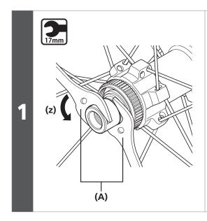
Use the spanner to loosen the lock nut on the double-lock section.
