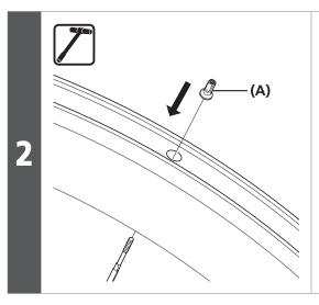
Attach the nipples using an inner nipple wrench.
