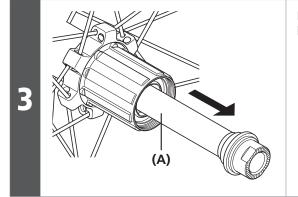
Pull out the hub axle from the freewheel body.
