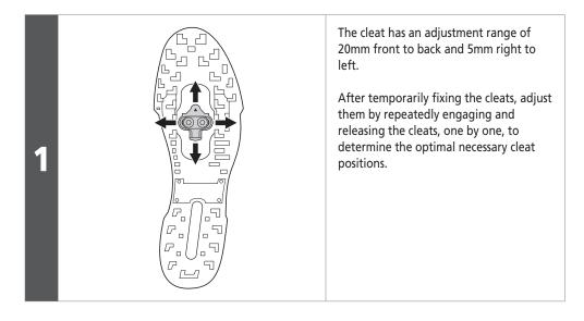
After the optimal cleat positions have been determined, firmly tighten the cleat mounting bolts with a 4mm hexagon wrench.
