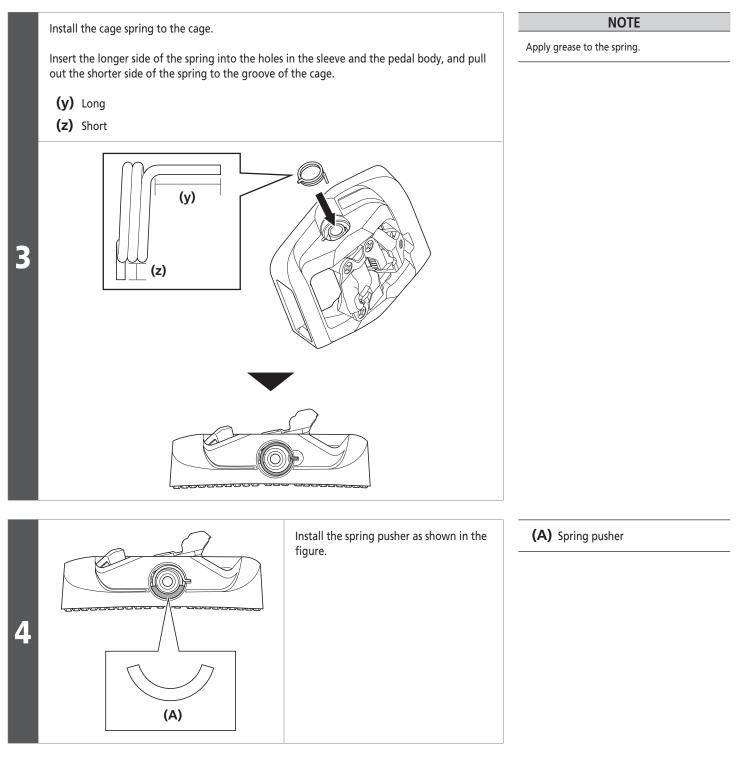
Replacing the cage
