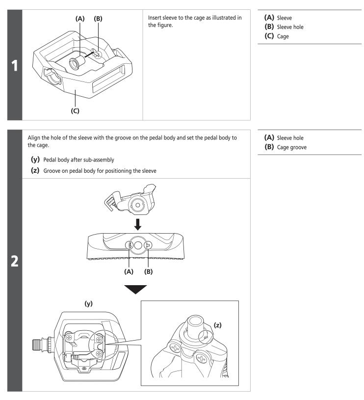
Replacing the cage
