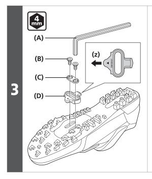
Position the cleat followed by the cleat adapter on to the sole of the shoe and then temporarily tighten them with the cleat mounting bolts.
