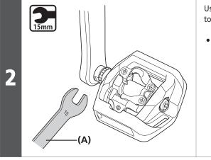
Use a 15mm spanner to install the pedals to the cranks.
