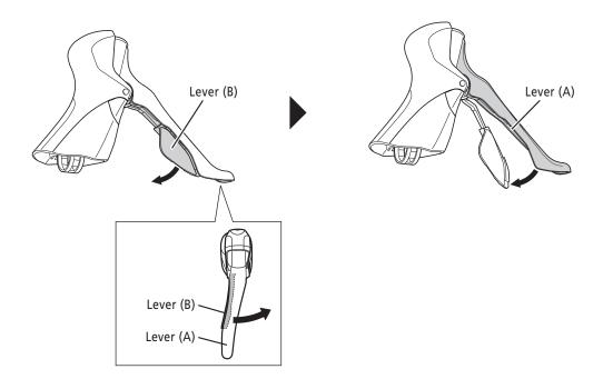
2. Hold the base of lever (A) and then return only lever (A) to the original position.
