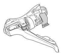
**3.** Pull out the inner end on the cable hook of the winding body.
