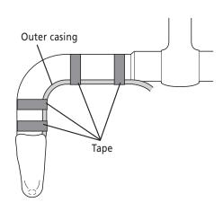
**7.** Then wrap the handlebar with handlebar tape.
