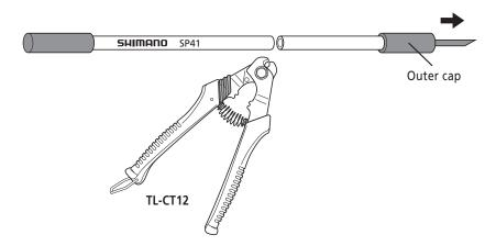
**2.** After cutting, expand the tip of the liner (\$\phi\$ 2.2 or more) with TL-CT12 or another narrow tool.
