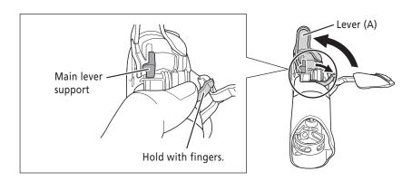
**3.** Rotate the main lever support in the direction of the arrow with a slotted screwdriver or an equivalent tool, and then remove the stopper.
