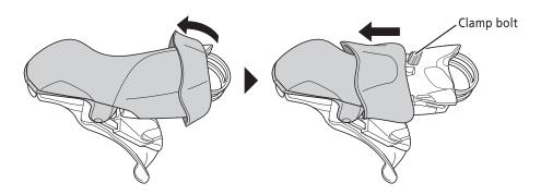
Use a 5 mm Allen key to tighten the clamp bolt.
