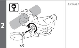
Remove the inner hole cap (A).
