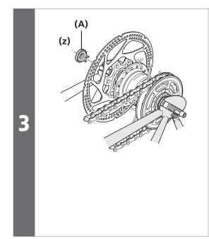
Place the non-turn washer (A) onto the left side of the hub axle from the outer side.
