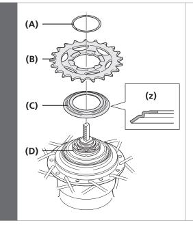
Place the right-hand waterproof cap C (C) onto the driver (D) on the right side of the hub body.
