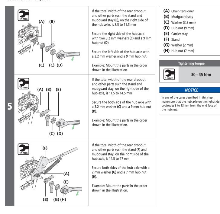
Installation of the bell crank type hub
