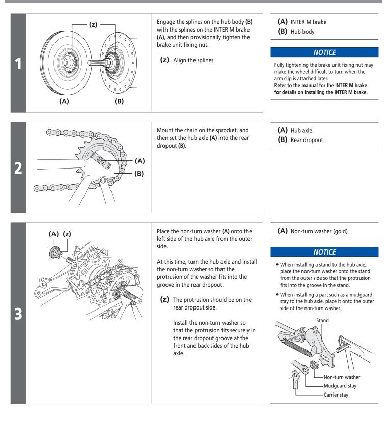
Installation of the bell crank type hub
