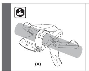
Secure the shift lever using the clamp screw (A).
