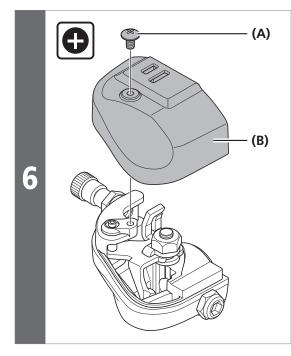
Tighten the bottom cover (B) with the bottom cover fixing screw (A).
