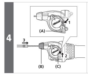
Hook the inner cable into groove in the pulley (A), and pull the inner cable so that the inner cable drum fits into the hole in the pulley (C).
