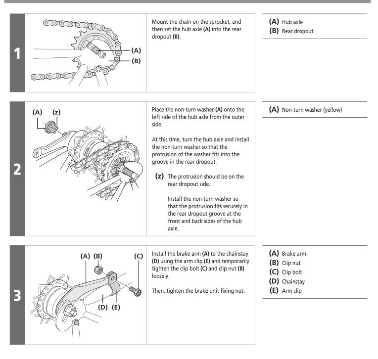
Installation of the bell crank type hub
