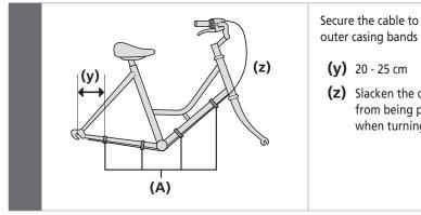
Secure the cable to the frame with the outer casing bands **(A)**.
