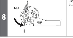
Turn the cable  $60^{\circ}$  counterclockwise and attach it to the hook **(A)**.
