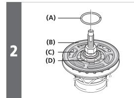
Install the CS-S500 sprocket (C) to the driver (D) on the right side of the hub body with the guard plate (B) facing outward, and secure it in place with the snap ring (A). (A) Snap ring
