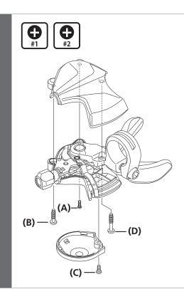
Remove the four mounting screws, and replace the cover.
