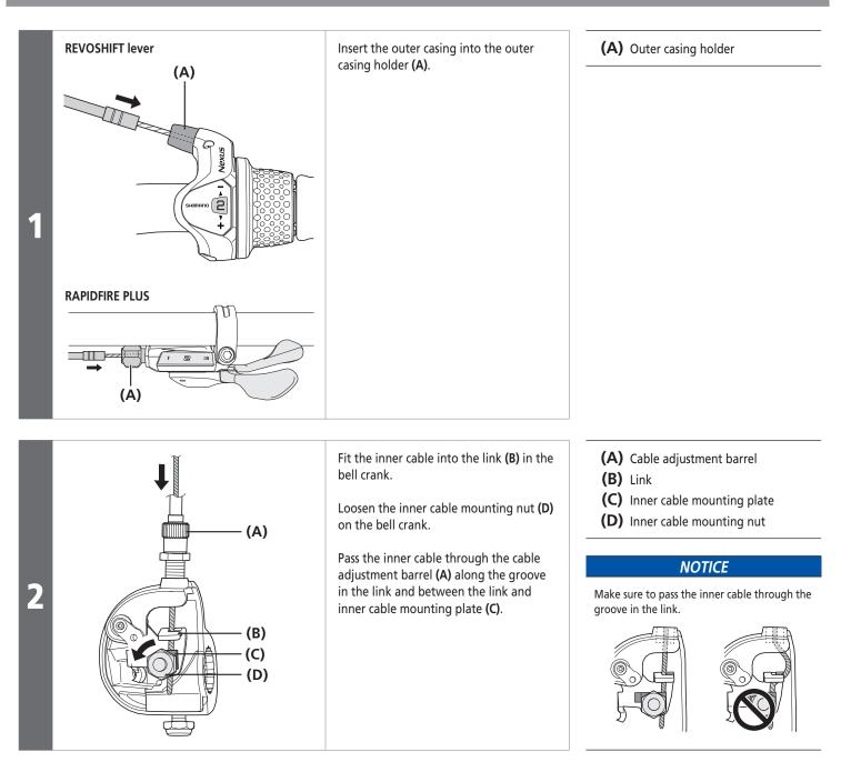
Installation of the bell crank type hub
