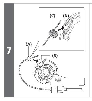
Bring the cable around to the cassette joint pulley (**B**), hold it so that the inner cable mounting nut (**A**) is facing outwards (towards the rear dropout), and then slide the flats part (**C**) of the inner cable mounting washer into the gap (**D**) in the pulley. (A) Inner cable mounting nut
