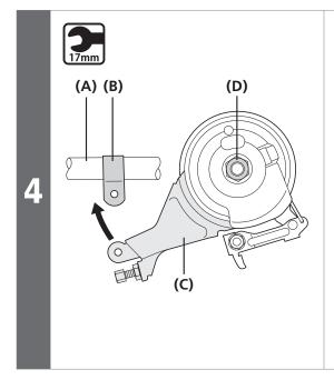
Install the brake arm (C) of the INTER M brake to the chainstay (A) using the arm clip (B) and temporarily tighten the clip bolt and clip nut loosely.
