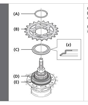
Place the right-hand waterproof cap B (C) onto the driver (D) on the right side of the hub body.
