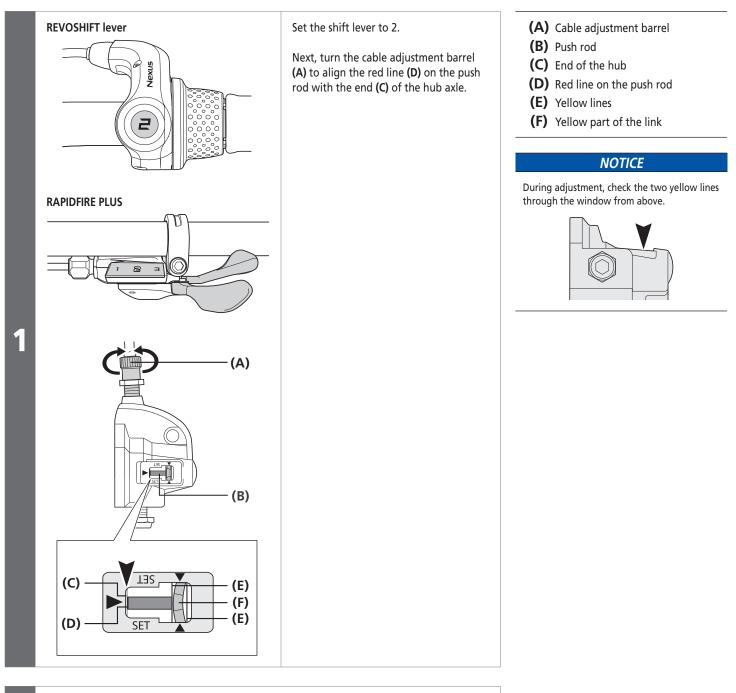
While turning the crank, move the shift lever from 3 to 1 then back to 3. Repeat this two or three times and check that the gears are being shifted. Move the shift lever from 1 to 2 again and make sure that the red line on the push rod is aligned with the end of the hub axle. If they are not aligned, perform readjustment.
