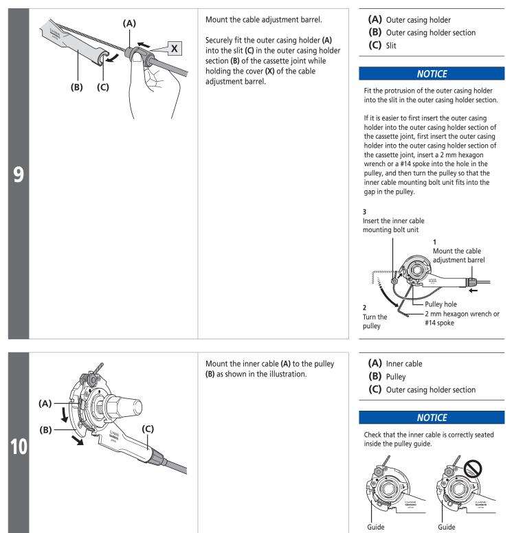
Installation of the cassette joint type hub
