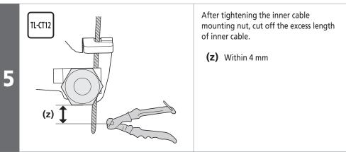
Installation of the bell crank type hub
