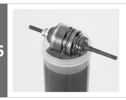
After lubrication is complete, reassemble by following the usual procedure.
