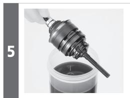
Let the excess oil drain off for approximately 60 seconds.
