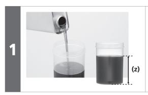
Fill the bottle with WB oil to a height of 95 mm.
