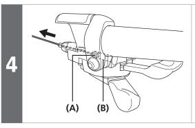
Pull the inner cable so that the inner cable drum fits into the hole in the winder unit.
