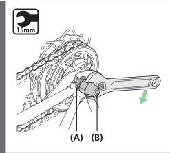
Take up the slack in the chain and secure the wheel to the frame with the cap nuts.
