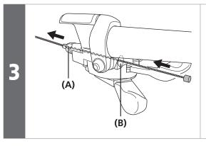
Insert the inner cable into the hole in the winder unit, and then pass it through the hole in the cable adjustment barrel.
