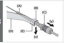
Remove the outer casing holder unit from the outer casing holder of the cassette joint (y).
