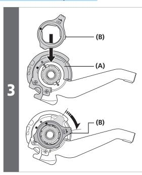
Secure the cassette joint to the hub with the cassette joint fixing ring.
