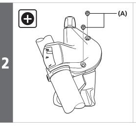
Secure the indicator unit with the two cover fixing screws.
