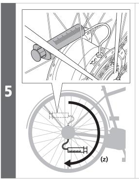
Insert the syringe between the spokes, and slowly turn the wheel forward until the oil port is facing down.
