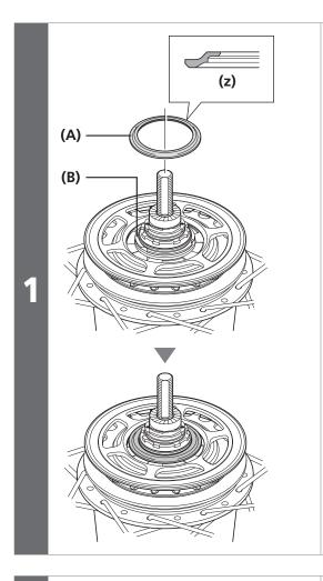
Install the driver cap to the driver on the right side of the hub body.
