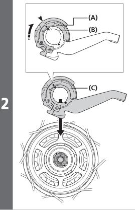
Turn the cassette joint pulley in the direction of the arrow in the illustration to align the red marks on the pulley and the bracket. With the cassette joint in this condition, install it so that the red mark on the cassette joint is aligned with the red mark on the right side of the hub body.
