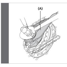
Disconnect the cable from the cassette joint when removing the rear wheel from the frame.
