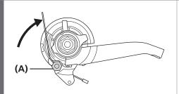
Turn the cable 60° counterclockwise and attach it to the hook.
