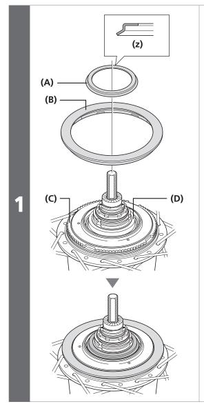
Install the chain guard to the right hand dust cap of the hub body, and then install right hand dust cap B to the driver.
