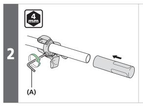
Mount the grip to the handlebar and secure the shift lever.
