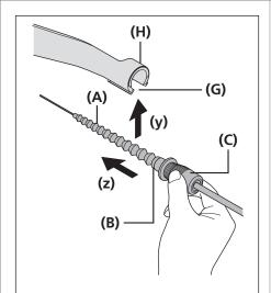
Set the inner cable in the pulley as shown in the illustration and, while holding the rubber cover, insert the rubber bellows of the inner cable into the slit in the cassette joint bracket (y) and securely set the outer casing holder unit into the outer casing holder of the cassette joint (z). Be careful not to damage the rubber bellows at this time.
