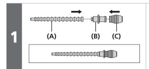
Install the rubber cover and rubber bellows to the outer casing holder unit.
