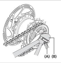
When not using the chain tensioner Mount the chain on the sprocket, then set the hub axle into the dropout.
