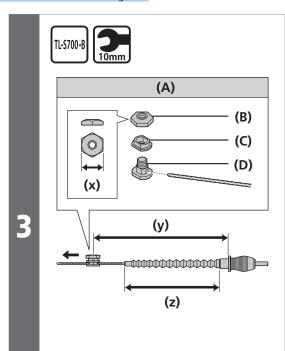
After checking that the end of the outer casing is sitting securely in the cable adjustment barrel of the shift lever, attach the inner cable fixing bolt unit to the inner cable.
