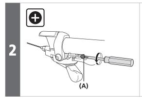
Loosen and remove the inner hole cap.
