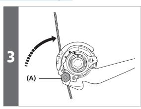
Turn the cable 60° counterclockwise and attach it to the hook.
