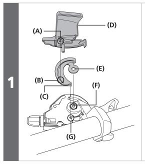
Check that the needle of the indicator is on the left side ( 11 position), and then install the indicator unit so that it is facing straight upward.
