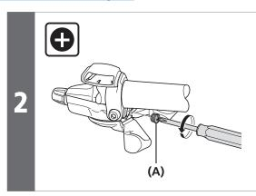
Loosen and remove the inner hole cap.
