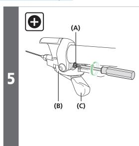
Screw in the inner hole cap as shown in the illustration until it stops.
