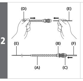
Wipe away any grease which may be on the inner cable and, while holding the end of the rubber bellows, pass the inner cable through. Be careful not to pierce the rubber bellows with the end of the inner cable at this time.
