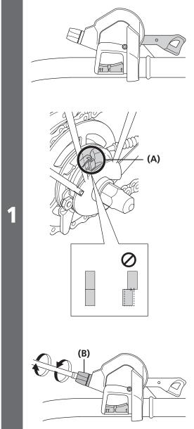
Set the shift lever from 11 to 6. Check to be sure that the yellow setting lines on the cassette joint bracket and pulley are aligned at this time.
