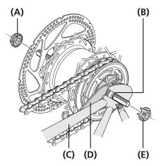
Place the non-turn washers onto the right side and left side of the hub axle.
