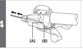
Pull the inner cable so that the inner cable drum fits into the hole in the winder unit.
