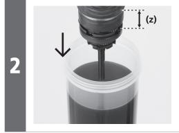
Immerse the internal unit into the oil from the left side. Immerse until the oil reaches up to ring gear unit 1.
