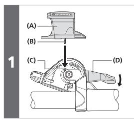
Check that the needle of the indicator is on the left side ( 8 position), and then install the indicator unit so that it is facing straight upward.
