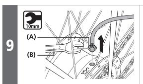
While being careful that the tube does not come off the syringe, remove the bleed nipple.
