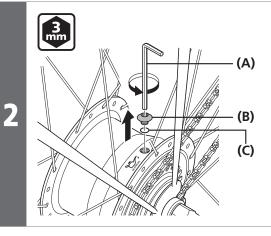
Remove the oil port screw and O-ring.
