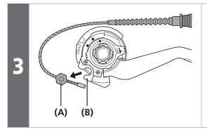
Remove the inner cable fixing bolt unit from the cassette joint pulley.
