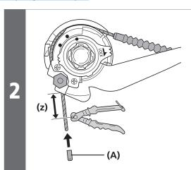
After adjusting the cassette joint, cut off the excess length of inner cable.
