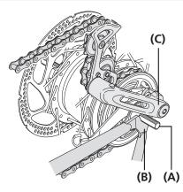
When using the chain tensioner Mount the chain on the sprocket, then set the hub axle into the dropout.
