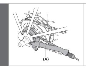
Disconnect the cable from the cassette joint when removing the rear wheel from the frame.
