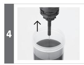
Remove the internal unit from the oil.
