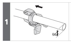
Mount the shift lever to the handlebar.
