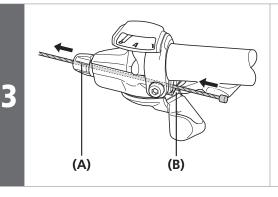
Insert the inner cable into the winder unit cable fixing groove, then pass it through the hole in the cable adjustment barrel
