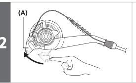
Press the lever of the pulley clockwise to loosen the inner cable. In the following steps 3 and 4, continue to work in this condition.
