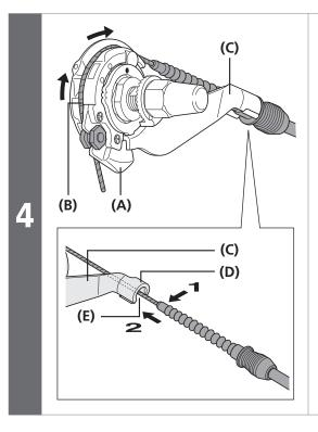
Attach the inner cable to the pulley as shown in the illustration, pass the inner cable through the slit in the cassette joint bracket, and then insert the end of the outer casing securely into the outer casing holder.
