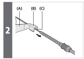
Pull the outer casing out from the outer casing holder of the cassette joint, and then remove the inner cable from the slit in the bracket.
