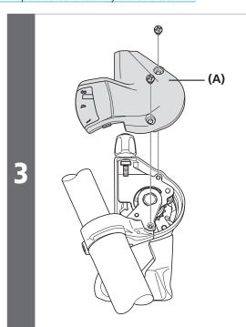
Remove the indicator unit as shown in the illustration.
