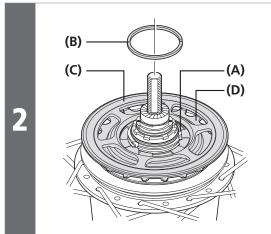
Install the CS-S500 sprocket to the driver on the right side of the hub body with the guard plate facing outward, and secure it in place with the snap ring.
