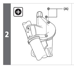
Loosen and remove the two cover fixing screws which are securing the indicator unit
