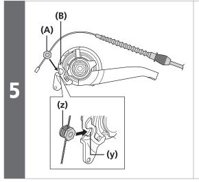
Bring the cable around to the cassette joint pulley, hold it so that the inner cable mounting nut is facing outwards (towards the dropout), then slide the flats part (z) of the inner fixing washer into the notch (y) in the pulley.
