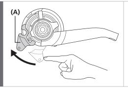
Turn the lever of the pulley clockwise. In the following steps 5 and 7, continue to work in this condition.
