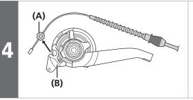
Remove the inner cable fixing bolt unit from the cassette joint pulley.
