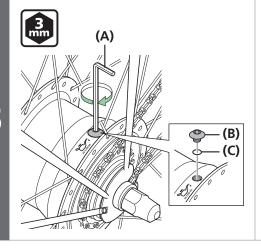
Install the O-ring and the oil port screw.
