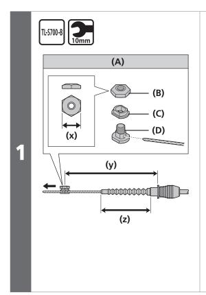
After checking that the end of the outer casing is sitting securely in the cable adjustment barrel of the shift lever, attach the inner cable fixing bolt unit to the inner cable.
