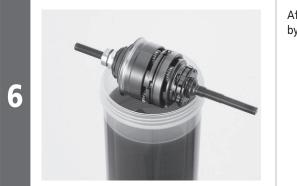
After lubrication is complete, reassemble by following the usual procedure.
