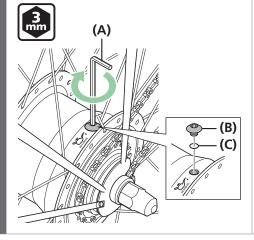
Install the O-ring and the oil port bolt.
