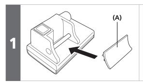
Install the rubber spacer to the system information display.
