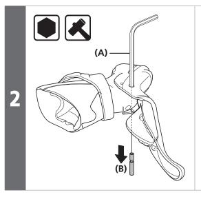
Insert a hexagon wrench or a similar tool into the hole in the lever axle, then tap it with a soft face mallet to push out the lever axle.
