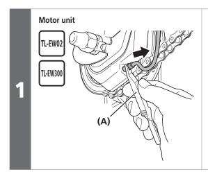
Remove the electric wire on the motor unit side.
