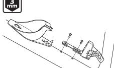
Use the included M4 screws to secure the short type.
