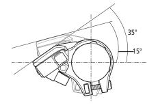
Installation of the dual control lever: Drop handlebar (ST-S705-R / BL-S705-L)
