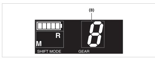
(B) Gear position/Adjustment level
