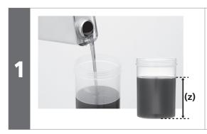
Fill the container with maintenance oil to a height of 95 mm.
