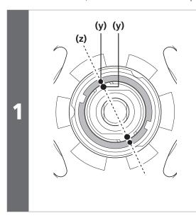
Check that the two • marks (y) (red) on the right side of the hub body are aligned.
