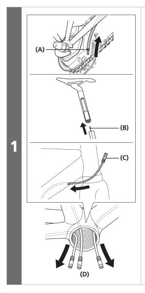
First, insert the electric wire for each of SC-5705, the battery mount, and the motor unit through the hole in the frame to the bottom bracket shell.
