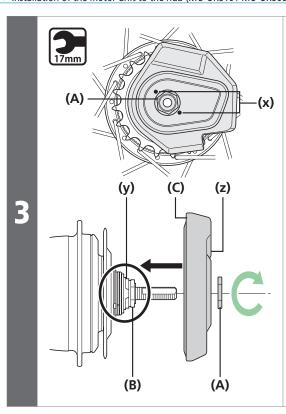
Install the motor unit to the hub so that the • mark (x) on the motor unit is aligned with the • mark (y) on the hub lock spacer.
