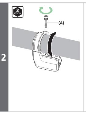
Adjust the angle of the system information display so that it is easy to see, and then use a 3 mm hexagon wrench to tighten the clamp bolt.
