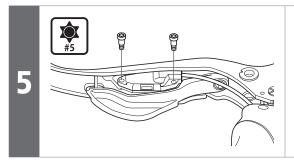
Return the switch unit to the setting position for the switch unit setting plate, and while pressing it by hand, operate the shifting switches [X/Y] once more and check that the switches turn on.
