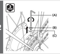
Remove the oil port bolt and O-ring.
