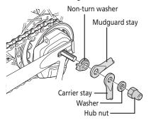
• When installing the hub to the frame, the chain guard may come off, so check that the chain guard is securely installed. If not properly installed, noise may be generated.
