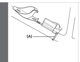
Tighten the bolt of the bottle cage to secure the battery mount.
