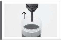
Remove the internal unit from the oil.
