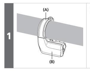
Insert the clamp band of the system information display into the handlebar.
