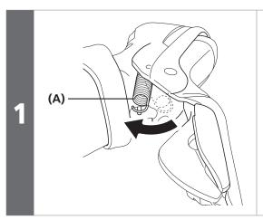
Assemble the bracket body and the lever body, and then attach the return spring.
