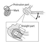
• Install the non-turn washer so that the protrusion fits securely in the rear dropout groove at the front and back sides of the hub axle.
