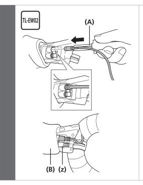
Open up the bracket cover and lift up the connector cover.
