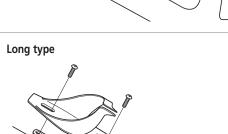
Use the bolts which are included with the bottle cage to secure the long type.
