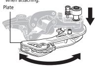
• If there is resistance when moving the lever switch to the ON position, the components are attached correctly.
