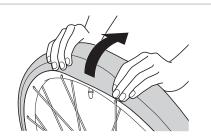
Grip the tire with both hands as shown in the illustration and insert the tire into the rim.
