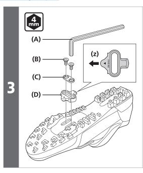
Position the cleat followed by the cleat adapter on to the sole of the shoe and then temporarily tighten them with the cleat mounting bolts. The cleats are compatible with both left and right pedals.
