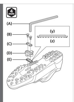
Position the cleat spacer, followed by the cleat, and then cleat adapter on to the sole of the shoe and then temporarily tighten them with the cleat fixing bolts.
