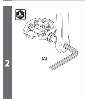
Use an 8 mm hexagon wrench to install the pedals to the cranks.
