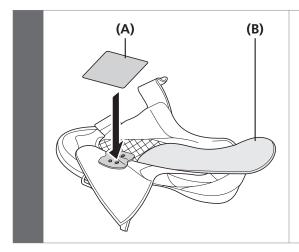
Remove the sockliner and attach the waterproof seal.
