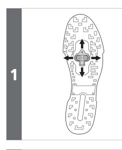
The cleat has an adjustment range of 20 mm front to back and 5 mm right to left.
