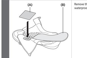
Remove the sockliner and attach the waterproof seal.
