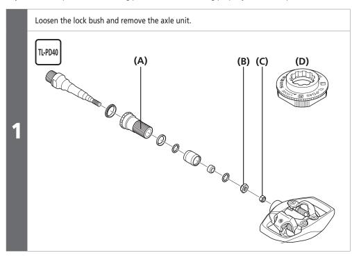
Use TL-PD63 or TL-PD33 Shimano original tool, or a 7mm or 10mm open wrench to turn the
