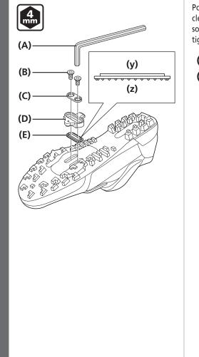
Position the cleat spacer, followed by the cleat, and then cleat adapter on to the sole of the shoe and then temporarily tighten them with the cleat fixing bolts.
