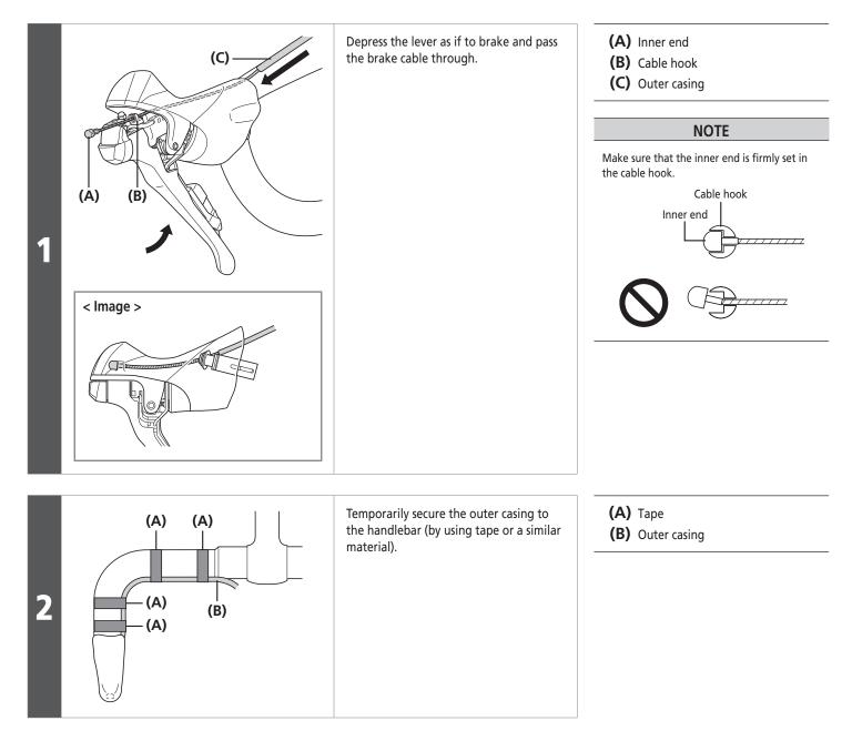
Installation of the cantilever brake
