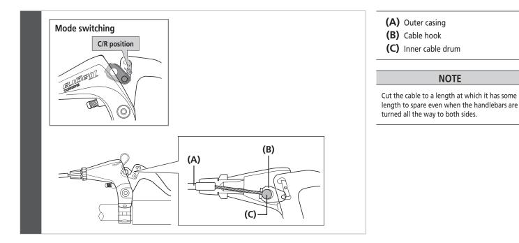
▶ Installation of the dual control lever (ST-7900/6700/5700/4600)
