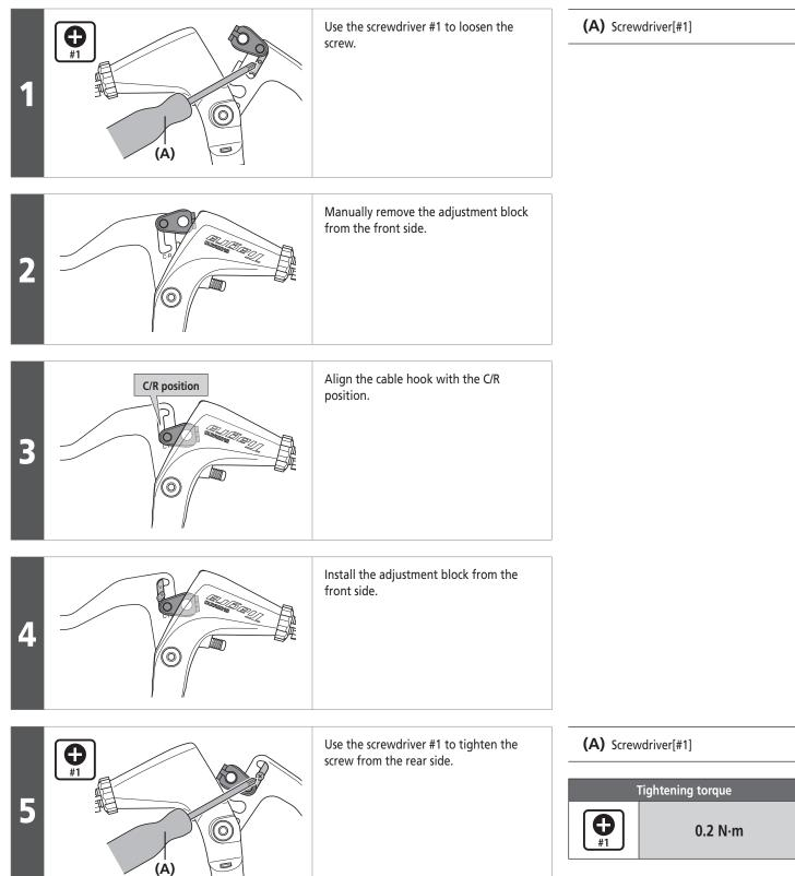
▶ Installation of the brake lever (BL-4700/4600/R780/R3000)
