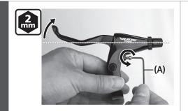
Turning counterclockwise causes the width to become wider.
