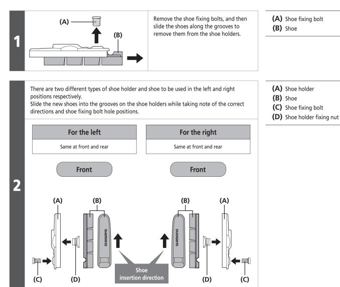
Use a 2 mm Hexagon wrench to tighten the shoe fixing bolts.
