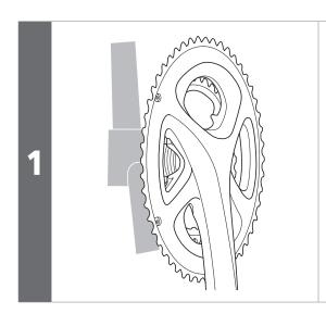
Fully insert the right crank arm unit until it touches the bottom bracket.
