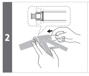
As shown in the illustration, hold down the flap with your fingers and push it in from the opposite side. (When pushed in, the flap opens.)
