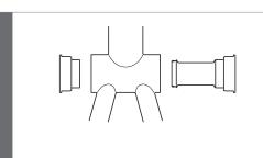
Use a bottom bracket compatible with a shell width of 86.5 mm.
