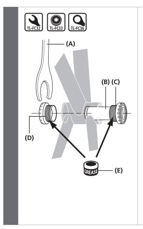
Grease the left- and right-hand cups and use the SHIMANO original tool to install the right-hand cup of the bottom bracket, the inner cover and the left-hand cup of the bottom bracket.
