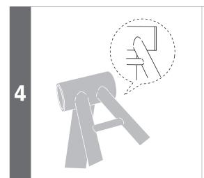
Check to confirm that there is no gap between the bottom bracket and the bottom bracket shell.
