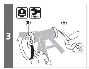
Press fit the bottom bracket by tightening with a spanner while making sure that the contact surface of the bottom bracket stays parallel to the contact surface of the bottom bracket shell.
