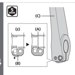
Push in the stopper plate and check that the plate pin is securely in place, and then tighten the screws of the left crank arm.
