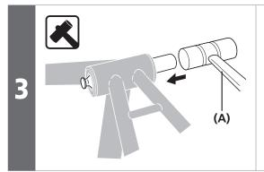
Tap the SHIMANO original tool with a soft face mallet until the end of the bottom bracket is ejected.
