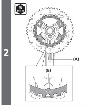
With the marked side of the smallest chainring facing inward, set the smallest chainring so that the alignment tab is positioned under the crank arm.
