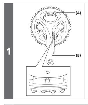
With the marked side of the largest chainring facing outward, set the largest chainring so that the chain drop prevention pin is positioned under the crank arm.
