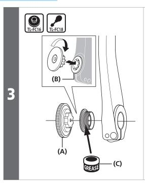
Use the SHIMANO original tool to tighten the cap.
