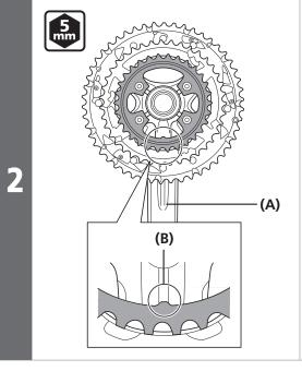
Set the middle chainring and the smallest chainring so that the marked sides face inward and the alignment tab on each chainring is positioned under the crank arm.
