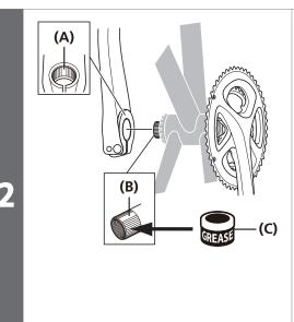
Set the wide groove area of the left crank arm into the axle of the right crank arm unit where the groove is wide.
