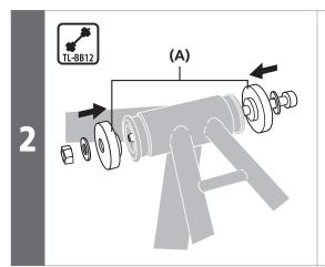
Insert the SHIMANO original tool into the bottom bracket.
