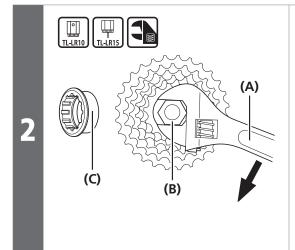
Set and tighten the lock ring.
