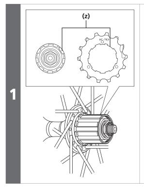
When setting the sprockets, set each one so that the surface that has the group mark faces outward and so that the wide groove area on the freewheel body is aligned with the wide groove area of the convex section on each sprocket.
