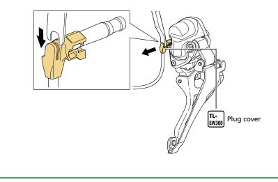
2. When checking of the connections is complete, temporarily remove the battery.
