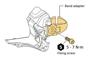
2. Tighten the support screw until it touches the band adapter.
