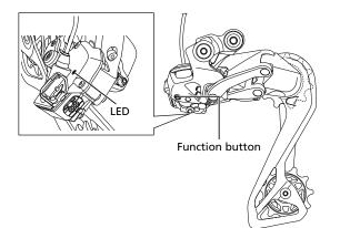
5. Shift the front derailleur and the rear derailleur to all gears to make sure that the chain does not contact the inner or outer plates.
