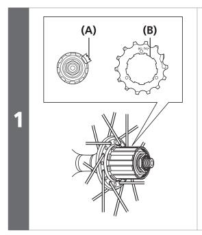
Place each sprocket with the marked side facing outward.
