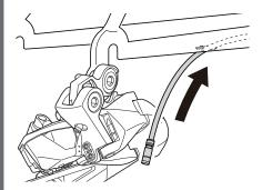
Electric wire for battery mount [In the case of an external battery (SM-BTR1)]
