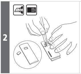
Hold the cut handlebar tape against the tool, and then cut out the holes for the switches while following the directions of the arrows on the tool.
