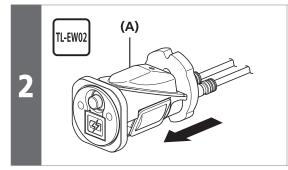
Connect the electric wires to junction A.
