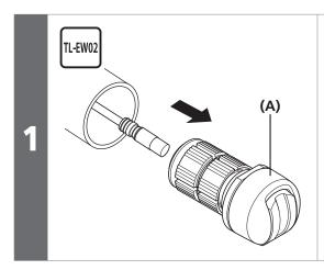
Connect the electric wire to the shifting switch.
