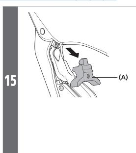
Remove the brake lever stopper.
