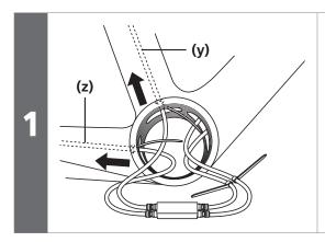
Pass the electric wires for the front derailleur and the rear derailleur through the seat tube and chainstay respectively.
