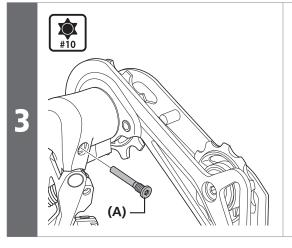
Using a Hexalobular[#10], remove the stopper bolt.
