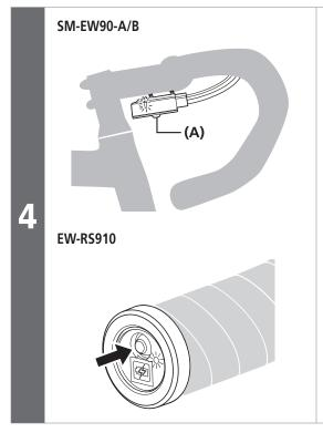
Press the button at junction A until the red LED turns off in order to switch from rear derailleur adjustment mode to gear shifting mode.
