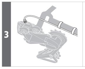
Temporarily secure the electric wire along the frame with tape, and connect it to junction B.
