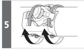
Rotate the zip tie until the square head on the zip tie fits into the notch in the adapter.
