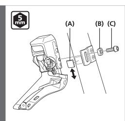
Attach the support plate where the support screw makes contact with the seat tube.
