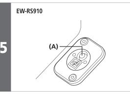
Press the button at junction A until the two LEDs turn off in order to switch from adjustment mode to gear shifting mode.
