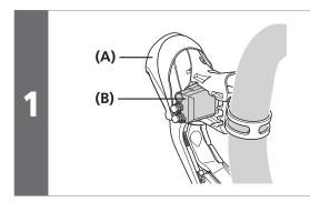
Pull back the bracket cover from the rear and lift up the connector cover.
