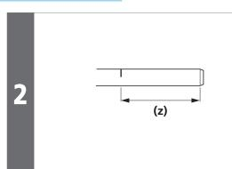
Put a mark on the brake hose beforehand as shown in the illustration so that you can check if the ends of the brake hose are secured to the hose mounts of the brake caliper and the dual control lever.
