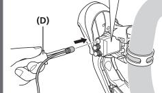
Use TL-EW02 to connect the connector of the electric wire to an E-TUBE port in the lever.
