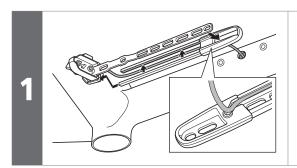
Set the electric wire for the battery mount into the groove in the electric wire cover for the battery mount.
