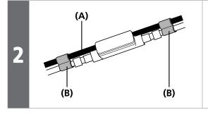
Secure the electric wires to the outer casing using the clips.
