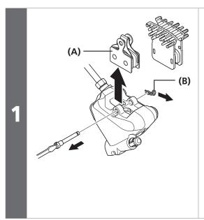
Remove the wheel from the frame, and remove the brake pads as shown in the illustration.
