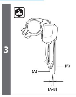
Use a 5 mm hexagon wrench to secure the outer plate so that the flat part of the plate is directly above the largest chainring and so that the rear edge of the chain guide is 0.5 - 1 mm in from the front edge.
