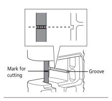
Check that the hose is secure and then attach the hose cutter.
