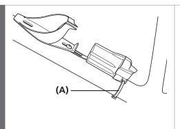
Tighten the bolt of the bottle cage to secure the battery mount.
