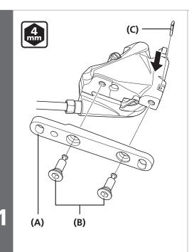
Attach the mount bracket to the brake caliper.
