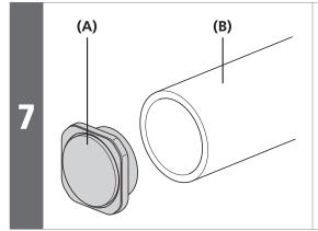
Insert the end cap into the handlebar end not fitted with junction A.
