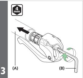
Install the brake lever to the handlebar by tightening clockwise with a hexagon wrench.
