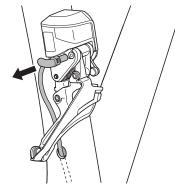
Electric wire for battery mount [In the case of a built-in battery (SM-BTR2/BT-DN110/BT-DN110-A)]
