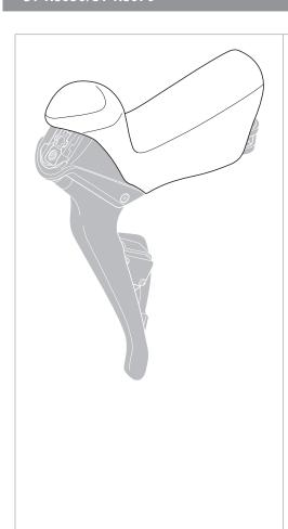
Fit the tabs on the bracket cover into the slots on the bracket unit.
