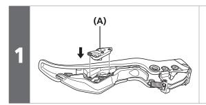
Attach the switch unit setting plate to the lever.
