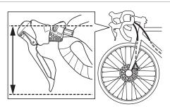
Adjust the position of the bleed screw so that its surface is parallel to the ground.
