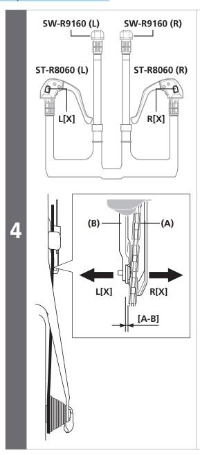
Operate shifting switch **R[X]** or **L[X]**.
