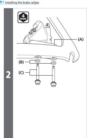
Attach the mount bracket to the frame.
