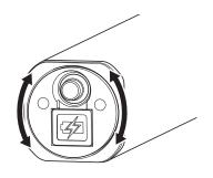
Do not tap junction A with a soft face mallet or similar tool when inserting it. Remove the release back sheet from the handle holders, and then install them to the handlebar.
