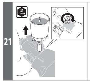
Remove the oil funnel and funnel adapter while still plugged with the oil stopper.
