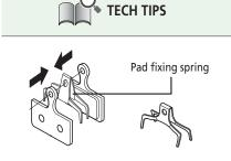
Install the pad fixing spring as shown in the illustration.
