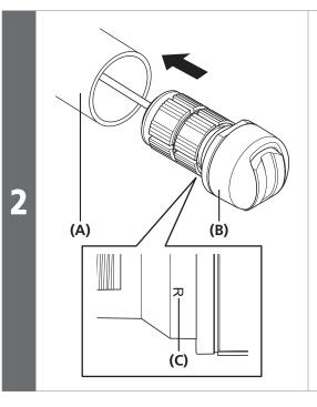
Check the marking (R or L) on the shifting switch and insert it into the end of the aero bar.
