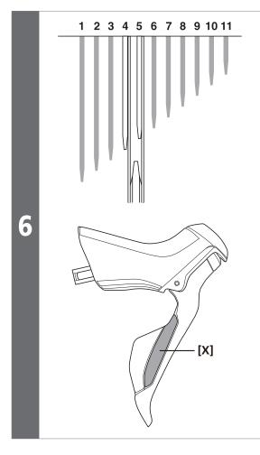
While turning the front chainwheel, operate shifting switch [X] to move the guide pulley toward the inside until the chain touches the 4th sprocket and makes a slight noise.
