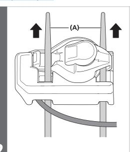
Pass zip ties through the adapter and shifting switch as shown in the illustration.
