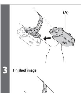
Slide SM-EW90 into the rail section of the hook to install it.
