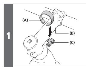
Attach to the stem using the band and hook included with SM-EW90.
