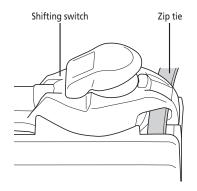
• When attaching the zip ties, make sure not to tie up the electric wire too.
