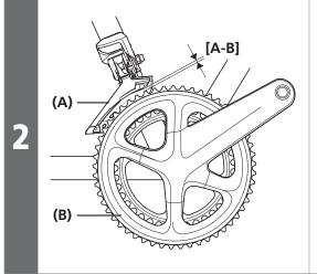
Adjust so that the clearance between the outer plate and the largest chainring is 1 - 3 mm.
