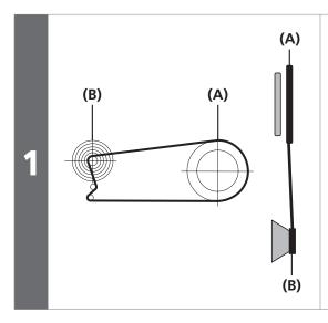
Set the chain on the largest chainring at the front and the smallest sprocket at the rear.
