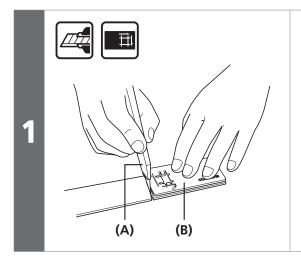
Use a utility knife or similar tool to cut the handlebar tape to the length shown in the illustration.
