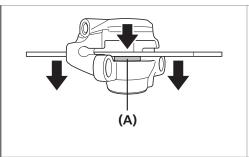
Use a flat-shaped tool to push the pistons straight back in as far as they will go, while being careful not to twist the pistons.
