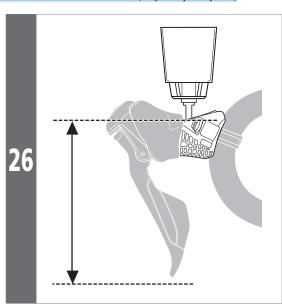
Make adjustments, such as changing the angle of the handlebar, so that the head of the bleed screw is parallel to the ground.
