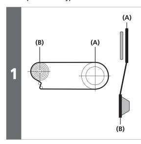
Set the chain onto the largest chainring at the front and the largest sprocket at the rear.
