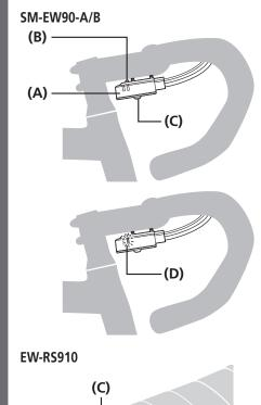
Press the button at junction A until the button LED illuminates in order to switch from gear shifting mode to adjustment mode.
