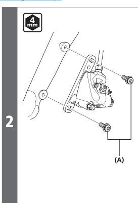
Temporarily attach the mount bracket to the frame.
