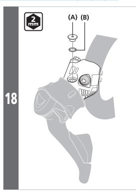
Remove the bleed screw and O-ring.
