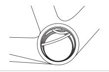
Set the electric wires so that only the electric wires for the front derailleur and the rear derailleur are visible inside the bottom bracket shell, and if any extra parts such as wire holders are protruding, push them back inside the frame.
