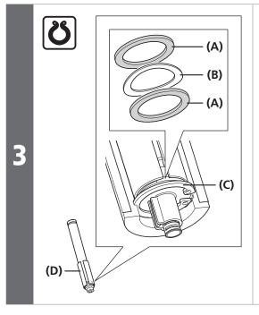
Mount a wave washer between two washers to the groove of the battery adapter, and fix them in place with a snap ring.
