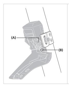
The high limit screw and the support bolt are close to each other.
