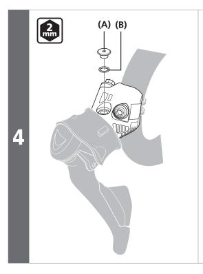
Remove the bleed screw and O-ring.
