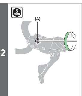
Use a 5 mm hexagon wrench to tighten the clamp bolt at the top of the bracket.
