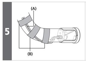
Secure the electric wires to the handlebar using tape or a similar material.
