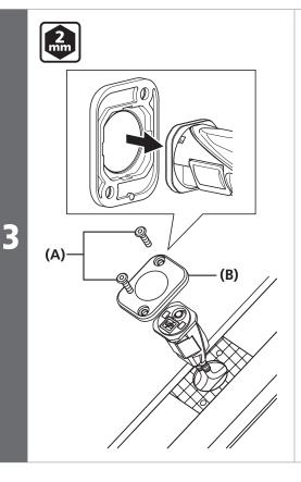
Insert junction A into the frame and attach the holder plate.
