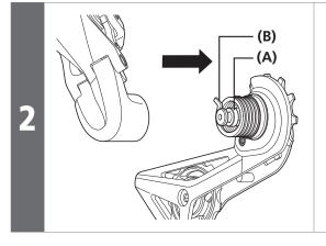
When reassembling, insert the end of the plate tension spring into the groove in the plate.
