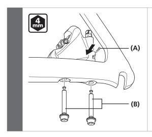
Attach the brake caliper to the frame.
