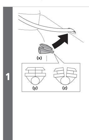
Install grommets in appropriate positions for the electric wires.
