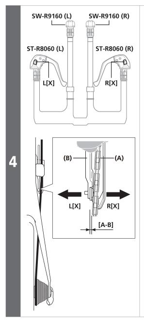
Operate shifting switch **R[X]** or **L[X]**.
