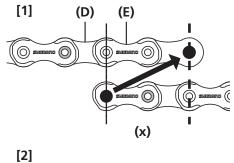
When mounting the chain, if the inner links and outer links match (as in [1]), set it to a length with 2 links added.
