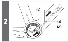
Pass the electric wires for junction A, the battery mount, and junction B through the down tube.
