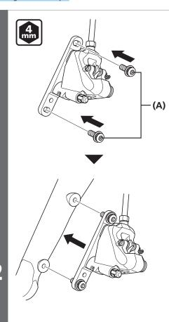
Insert the brake caliper mounting bolts A into the holes in the mount bracket first and then temporarily attach the mount bracket to the frame, as in the illustration.
