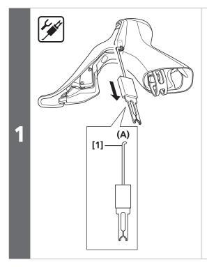
Use the SHIMANO original tool which is sold separately to remove the snap ring.
