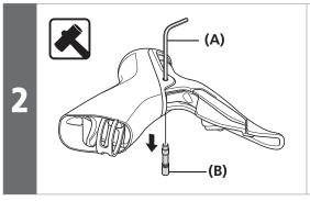
Insert a hexagon wrench or a similar tool into the hole in the lever axle, and then tap it with a soft face mallet to push out the lever axle.
