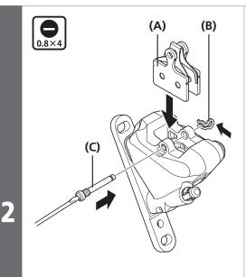
Install the new brake pads and bolts.
