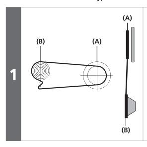
Set the chain on the smallest chainring at the front and the largest sprocket at the rear.
