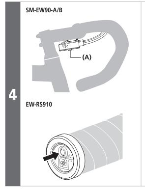
Press the button at junction A until the red LED turns off in order to switch from adjustment mode to gear shifting mode.
