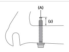
Insert the brake caliper mounting bolts C into the frame mount area, and make sure that the lengths of the protruding sections of the bolts are 13 mm.
