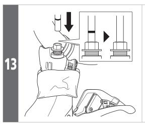
Insert the brake hose into the joint component until the mark on the hose is hidden.
