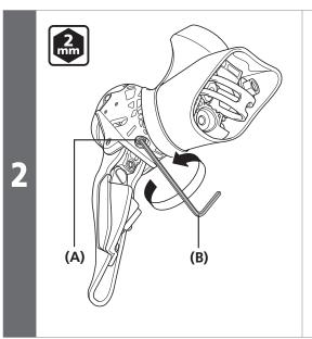
Turn the free stroke adjustment screw to adjust the stroke.
