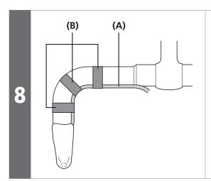
Temporarily secure the brake hose to the handlebar (by using tape or similar material).
