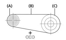
Mount the chain on to the largest sprocket at the rear and the largest chainring at the front.
