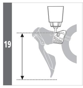
Make adjustments, such as changing the angle of the handlebar, so that the head of the bleed screw is parallel to the ground.
