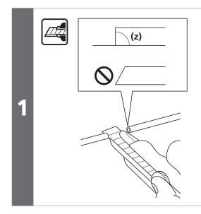
Use a utility knife or other cutting tool to cut the brake hose.
