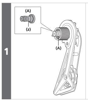
Apply grease to the plate axle.
