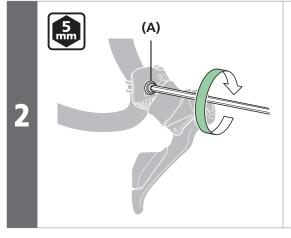
Use a 5 mm hexagon wrench to loosen the clamp bolt at the upper section of the bracket then tighten it after setting it on the handlebar. (A) Clamp bolt
