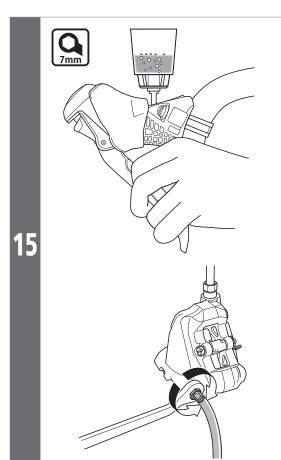
With the brake lever depressed, open and close the bleed nipple in rapid succession (for approximately 0.5 seconds each time) to release any air bubbles which may be in the brake calipers.
