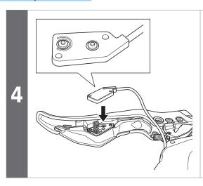
Place the switch unit onto the mounting surface of the setting plate.
