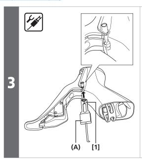
Use part [1] of the SHIMANO original tool to install the snap ring.
