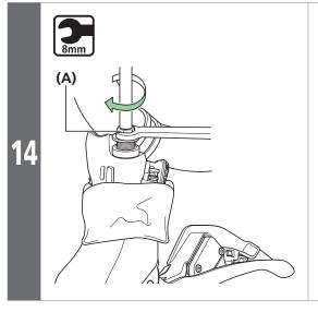
Tighten the flare nut with flange with an 8 mm spanner while pushing in the brake hose.
