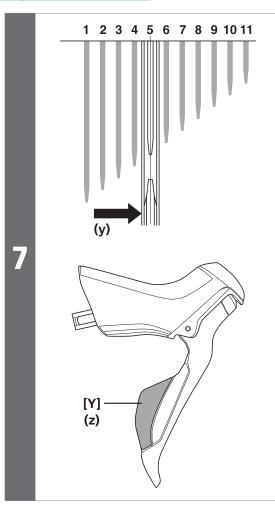
Next, operate shifting switch [Y] 4 times to move the guide pulley toward the outside by 4 steps to the target position.
