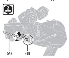
Shift the rear derailleur to the largest sprocket, and then tighten the low limit stopper bolt until it just touches the left link.
