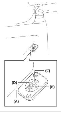
Press the button at junction A until the button LED illuminates in order to switch from gear shifting mode to adjustment mode.
