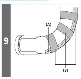
Secure the dummy wires to the handlebar using tape or a similar material.
