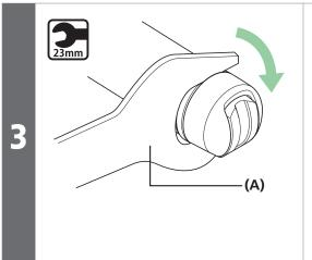
Hold the end of the shifting switch and tighten the nut part with a hub spanner.
