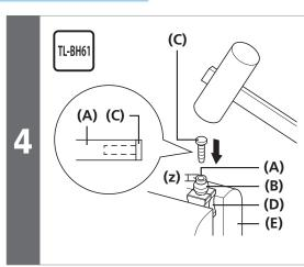
Use a tapered tool to smooth out the inside of the cut end of the brake hose, and mount the connector insert.
