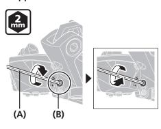
Shift to the smallest sprocket, and then tighten the top-side stopper bolt until it touches the left link at the position where the rear derailleur stops.
