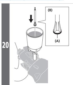
Plug the oil funnel with the oil stopper so that the O-ring mounted side is facing downward.
