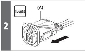
Connect the electric wires to junction A.
