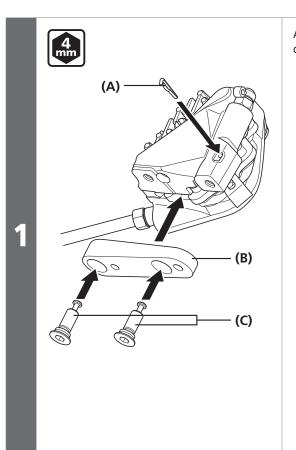
Attach the mount bracket to the brake caliper.
