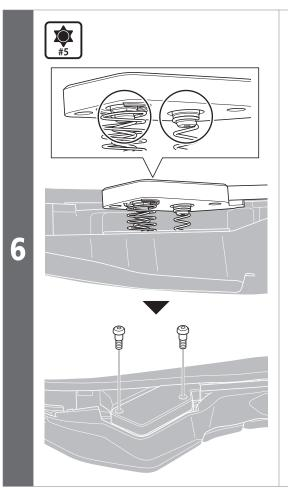
Make a gap between the switch unit and the setting plate and check that the end of the rubber on the switch unit is on the button.
