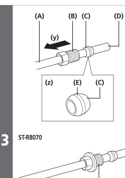
Pass the brake hose through the flare nut and olive as shown in the figure.
