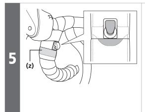
Wind on the handlebar tape.
