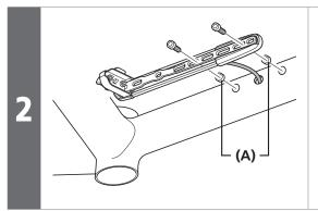
Place the accessory spacers in between the battery mount and the frame and then secure them by tightening the bolts. (A) Spacer
