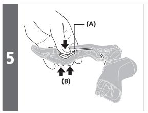
Press the switch unit by hand so that the switch springs go into the grooves in the buttons, and then push the shifting switches [X] and [Y] in as far as they will go.
