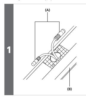
Pull out the electric wires through the hole in the frame as shown in the illustration.
