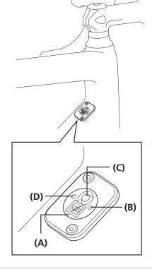
Press the button at junction A until the button LED illuminates in order to switch from gear shifting mode to adjustment mode.
