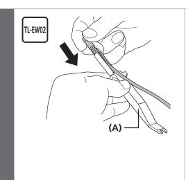
Set so that the projection on the connector is aligned with the groove on the narrow end.
