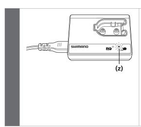
Remove the battery from the battery charger, disconnect the power plug of the battery charger from the electrical outlet, and then repeat the charging operation.
