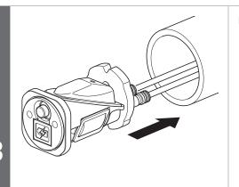
Insert junction A into the handlebar.
