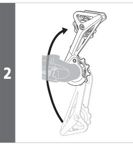
Turn the plate to loosen the plate tension spring as shown in the illustration.
