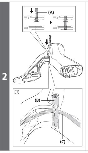
Align the axle holes, and then press-fit the lever axle.
