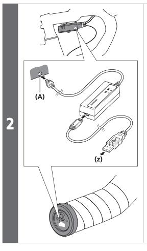
Connect the charging cable of the charger to the junction A.
