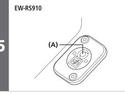
Press the button at junction A until the two LEDs turn off in order to switch from adjustment mode to gear shifting mode.
