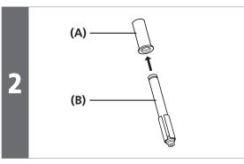
Insert internal battery into the collar from the bottom of seat post.
