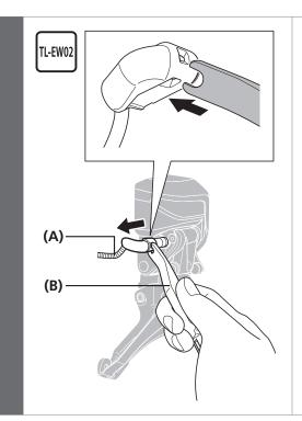
Insert the tips of the wider end of the TL-EW02 into the two holes on the plug cover, then remove the electric wire.
