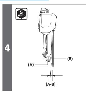
Use a 5 mm hexagon wrench to secure the outer plate so that the flat part of the plate is directly above the largest chainring and so that the rear edge of the chain guide is 0.5 - 1 mm in from the front edge.
