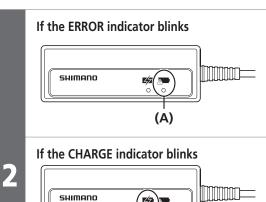
If the ERROR indicator blinks, the ambient temperature during charging may fall outside the operating temperature limits.
