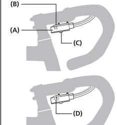
Press the button at junction A until the button LED illuminates in order to switch from gear shifting mode to adjustment mode.
