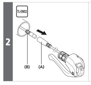
Connect the electric wire to the connector (female) extending from the lever.
