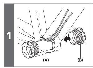
When installing the inner cover to the bottom bracket shell, make sure that the electric wires for the front derailleur and the rear derailleur pass over the top of the inner cover.
