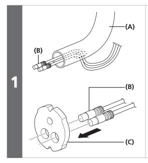
Route the electric wires through the hole in the handlebar as shown in the illustration.
