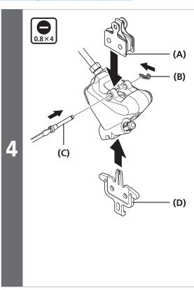
Install the new brake pads, the bolt, and the pad spacer (red).
