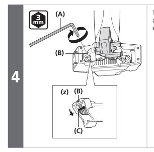
Turn the adjustment bolt on the pedal to adjust the spring tension to the strongest setting.
