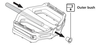
6. Remove old grease and apply an appropriate amount of new grease to the inner bush and outer bush.
