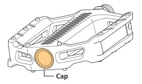
2. Use the TL-PD400 SHIMANO original tool to turn the cone to adjust the bearing preload.
