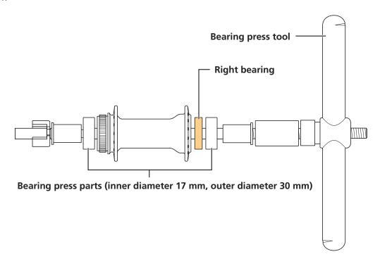
(2) Turn the handle of the bearing press tool, and insert the right bearing as far as it will go.
