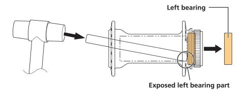
4. The unit can be disassembled as shown in the figure. Apply grease to the indicated parts.
