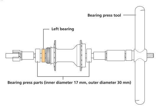
(2) Turn the handle of the bearing press tool, and insert the left bearing as far as it will go.
