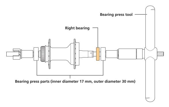
(3) Turn the handle of the bearing press tool, and insert the right bearing as far as it will go.
