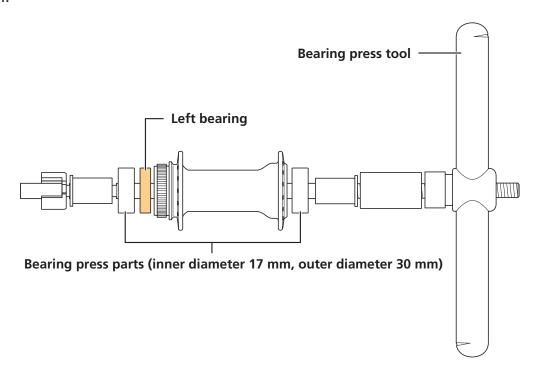
(3) Turn the handle of the bearing press tool, and insert the left bearing as far as it will go.
