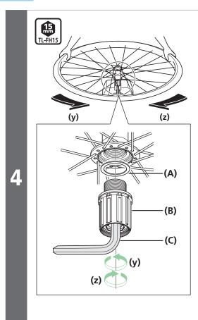
After removing the hub, remove the freewheel body fixing bolt (inside the freewheel body), and then replace the freewheel body.
