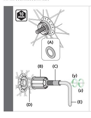
After removing the hub axle, remove the freewheel body fixing bolt (inside the freewheel body), and then replace the freewheel body.
