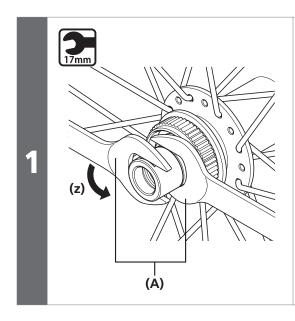
Use the spanner to loosen the lock nut on the double-lock section.
