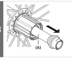
Pull out the hub axle from the freewheel body.
