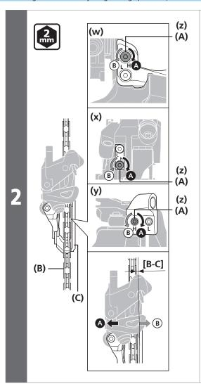
Adjust the position of the chain guide with the top adjustment bolt.
