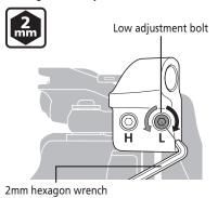
When adjustment is complete, tighten the clamp bolt.
