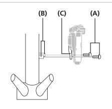
Secure with bottom bracket mount fixing bolts.
