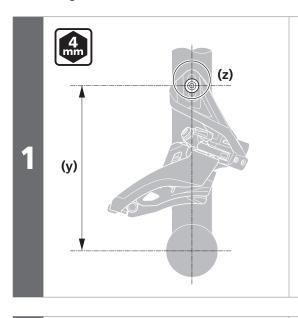
Temporarily attach the front derailleur to the frame.
