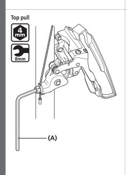
Use a spanner or a hexagon wrench to tighten the cable-fixing bolt.
