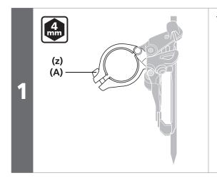
Temporarily attach the clamp bolt.
