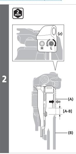
Adjust the low adjustment bolt and align the flat portion of the chain guide outer plate parallel to the flat surface of the largest chainring.
