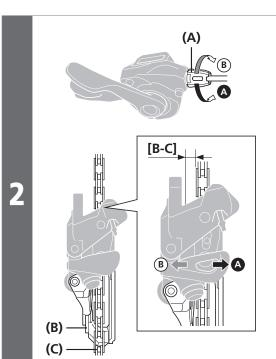
Adjust the position with the cable
