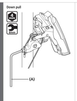
Use a spanner or a hexagon wrench to tighten the cable-fixing bolt.
