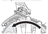
When performing a readjustment etc., without a pro-set alignment block, align the flat surface of the largest chainring using the low adjustment bolt.
