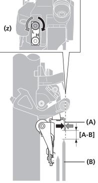
Adjust the low adjustment bolt and align the flat portion of the chain guide outer plate parallel to the flat surface of the largest chainring.
