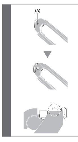
Align the rubber pad B mounting hole of the chain guide with the protrusion of rubber pad B.
