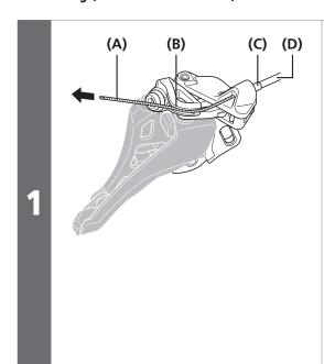
Adjust the shifting lever to the low position.
