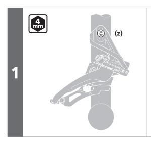
Temporarily attach the front derailleur to the frame.
