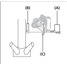
Secure with bottom bracket mount fixing bolts.
