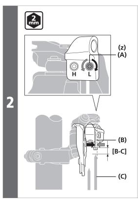
Adjust the low adjustment bolt and align the flat portion of the chain guide outer plate parallel to the flat surface of the largest chainring.
