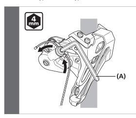
Use a hexagon wrench to tighten the cable-fixing bolt.
