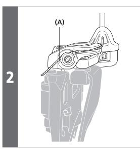
Pass the inner cable through along the cable guide on the top of the fixing bolt.
