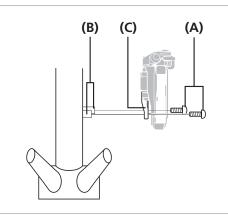
Install the front derailleur with bottom bracket mount fixing bolts.
