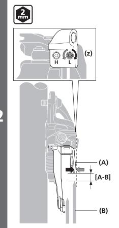
Adjust the low adjustment bolt and align the flat portion of the chain guide outer plate parallel to the flat surface of the largest chainring.
