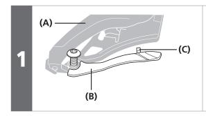
Temporarily attach the chain catcher to the chain guide.
