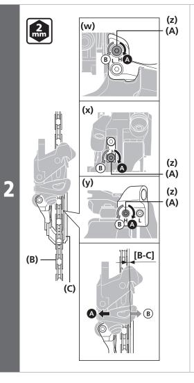
Adjust the position of the chain guide with the top adjustment bolt.
