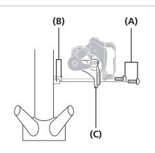
Secure with bottom bracket mount fixing bolts.
