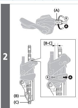
Adjust the position with the cable adjuster.
