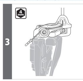
Fix the inner cable with a cable-fixing bolt.
