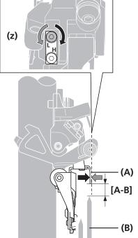
Adjust the low adjustment bolt and align the flat portion of the chain guide outer plate parallel to the flat surface of the largest chainring.
