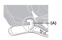
Securely attach the arm of the chain catcher as shown in the illustration.
