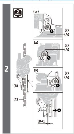
Adjust the position of the chain guide with the low adjustment bolt.
