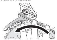
When adjustment is complete, tighten the clamp bolt.
