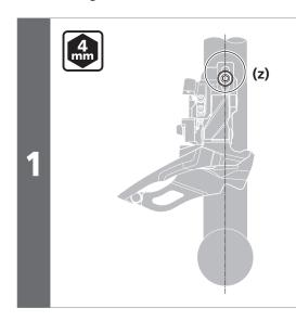
Temporarily attach the front derailleur to the frame.
