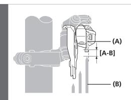
Align the flat portion of the chain guide outer plate in parallel with the flat surface of the largest chainring.
