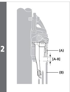
Align the flat portion of the chain guide outer plate in parallel with the flat surface of the largest chainring.
