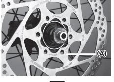
Place the disc brake rotor on to the hub, and then temporarily fix it in place by tightening the disc brake rotor fixing bolts.
