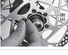
Wear gloves and turn the disc brake rotor clockwise with some force.
