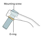
4. Attach the brake lever to the handlebar.
