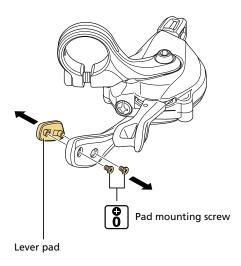
2. Replace the lever pad, then tighten the pad mounting screws.
