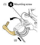
2. Temporarily attach the seat post lever to the clamp band.
