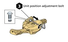
6. Tighten the unit position adjustment bolt.
