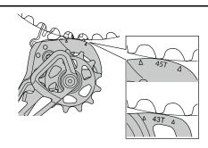
(C) Set the distance between the tip of the highest tooth on the largest sprocket and the center of the guide pulley as listed in the table.
