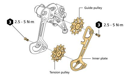
(2) Insert a hexalobular wrench into the outer plate and check the friction torque.
