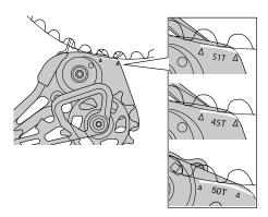
(B) Align the contour of the outer plate and the tip of the highest tooth on the largest sprocket between the arrows on the inner side of the outer plate.
