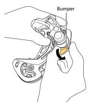
2. Install a new bumper by sliding it on from the side as shown in the figure.
