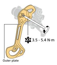
(3) Install the inner plate, guide pulley, and tension pulley.
