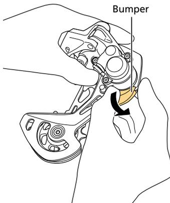
2. Install a new bumper by sliding it on from the side as shown in the figure.
