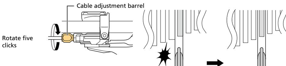
5. Operate the shift lever to change gears while turning the crank, and check that no noise occurs in any of the gear positions.
