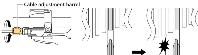
4. The best setting is achieved when the cable adjustment barrel is turned five clicks in the clockwise direction.
