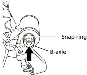
2. **Push the threaded portion of the B-axle against the stopper plate and use the hexagon wrench to unthread the B-axle from the stopper plate.**
