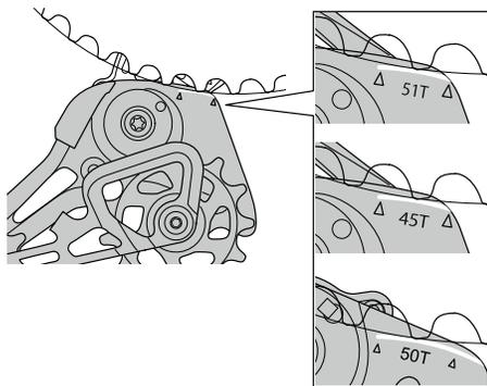
(B) Align the contour of the outer plate and the tip of the highest tooth on the largest sprocket between the arrows on the inner side of the outer plate.
