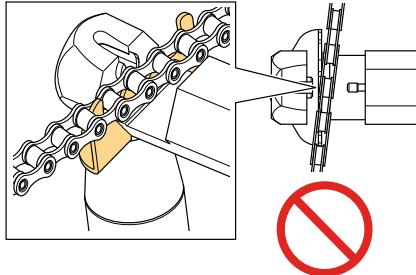
**2. Turn the handle of the chain cutter to push out the pin.**
