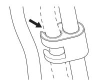
EZ cable clamp A: Cable outside diameter 5 mm
