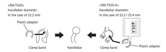
Widen the clamp band of the bracket, install it to the handlebar and then provisionally secure it.
