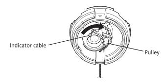
$\boldsymbol{5.}$  Install the indicator, lens cover, lens and cover in that order.
