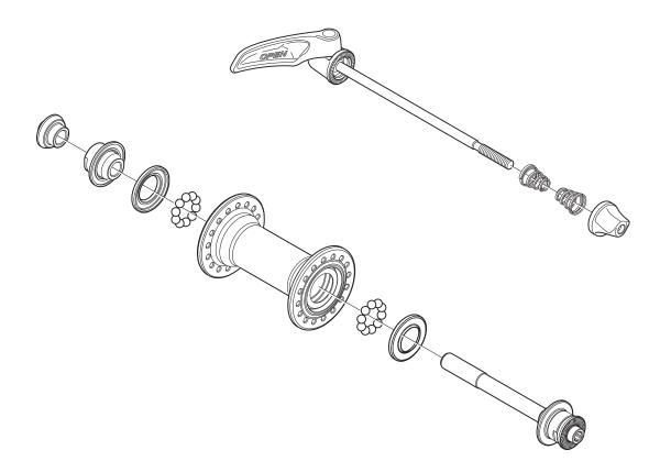
Pull out the hub axle by following the procedure shown in the illustration. Disassembly from the right side is not possible.
