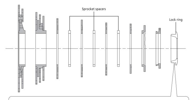
• For installation of the HG sprockets, use the SHIMANO original tool TL-LR15/LR10 to tighten the lock ring.
