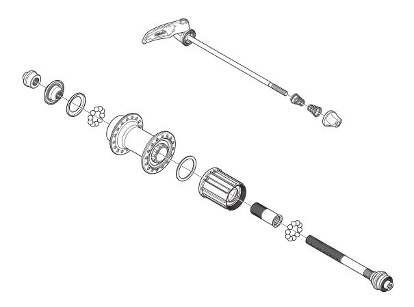
Pull out the hub axle by following the procedure shown in the illustration. Disassembly from the right side is not possible.
