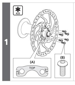
Install the disc brake rotor and rotor lock washers to the hub and tighten the screws.
