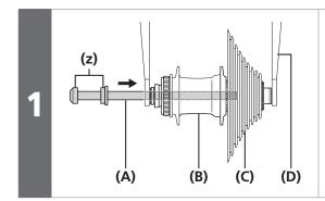
Install the sprockets to the freehub, place the freehub onto the frame and pass the hub axle through it.
