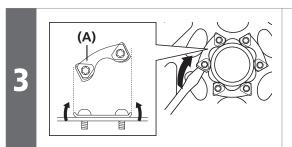
Use a slotted screwdriver or similar tool to bend the edges of the tightening plate over the heads of the screws.
