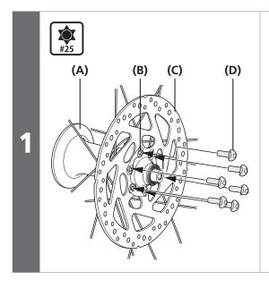
Install the disc brake rotor and the disc brake rotor tightening plate to the hub, and then install and tighten the screws. **(A)** Hub
