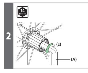
After removing the hub axle, remove the freewheel body fixing screw (inside the freewheel body).
