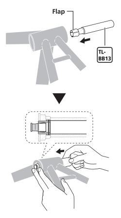
**2.** Tap the SHIMANO original tool with a soft face mallet to push out the cup.
