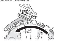
When adjustment is complete, tighten the clamp bolt.
