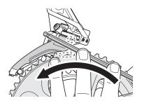
When performing a readjustment etc., without a pro-set alignment block, align the flat surface of the largest chainring using the low adjustment bolt.
