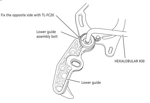
**3.** When installing a lower guide, reverse the procedure.
