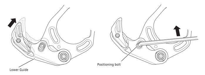
2. Fix the nut with TL-FC20, loosen the lower guide assembly bolt with Hexalobular #30 to remove it, and replace the lower guide with a new one.
