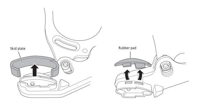
**3.** When installing a skid plate, reverse the procedure. Fit the convex part of the rubber pad into the concave part of the lower guide and after attaching the skid plate, tighten the guide fin using 2.5mm allen key.
