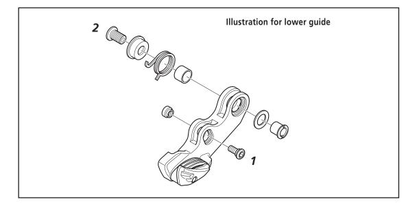
**1.** Fix the nut with a flat blade screwdriver and loosen the positioning bolt with a 4-mm Allen key. After that, remove the positioning bolt while holding up the lower guide.
