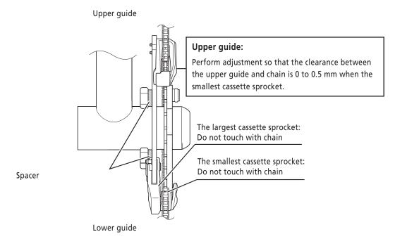
**3.** Adjust the height of the guide to leave a 0.5 to 1-mm clearance between the upper guide and the narrowest part of the guard, and Upper guide secure the guide to the backplate.
