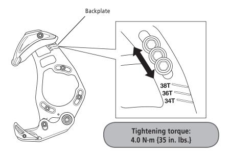
**4.** After installing the chain, with the cassette sprocket in the lowest position and the rear suspension stretched, rotate the backplate to leave a 0 to 1-mm clearance from the rubber band, and fix the backplate with the clamp bolt.
