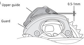
\* Adjust the height of the guide to the reading of the backplate scale when not using a guard.
