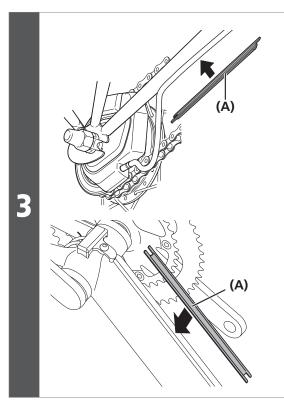
Install the electric wire cover/cord cover onto the frame.
