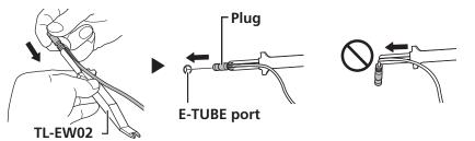
• When disconnecting the EW-SD50, lift the TL-EW02 straight up as indicated in (A), or use the TL-EW02 as a lever as indicated in (B).
