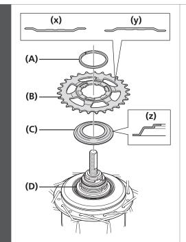
Place right-hand dust cap onto the driver on the right side of the hub body.
