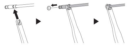
• When disconnecting the EW-SD300, the method below can also be used. Lift the TL-EW300 straight up as indicated in (A), or use the TL-EW300 as a lever as indicated in (B).
