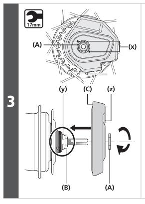
Install the motor unit to the hub so that the  $\bullet$  mark (x) on the motor unit is aligned with the  $\bullet$  mark (y) on the hub lock spacer.
