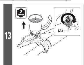
Remove the oil funnel while it is still plugged with the oil stopper, and then attach the O-ring to the bleed screw and tighten it while letting oil flow out to make sure that there are no air bubbles remaining inside the reservoir tank.
