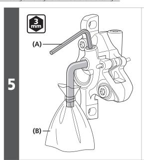
Tie the supplied tube and bag with rubber bands, set a 3mm hexagon wrench as shown in the illustration, and connect the tube to the bleed boss.
