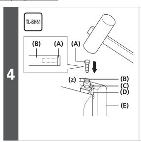
Use a tapered tool to smooth out the inside of the cut end of the hose, and then place in the connector insert.
