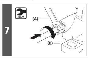
While pushing the brake hose, tighten the connecting bolt.
