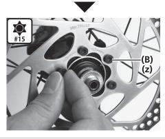
Place the disc brake rotor on to the hub, and then temporarily fix it in place by tightening the disc brake rotor fixing bolts.
