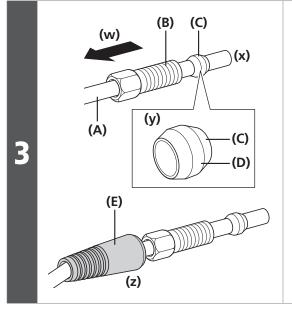
Pass the brake hose through the connecting bolt and olive.
