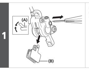
Remove the wheel from the frame, and remove the brake pads as shown in the illustration.
