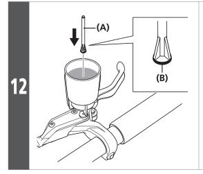
Plug the oil funnel with the oil stopper so that the O-ring mounted side is facing downward.
