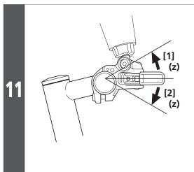
Set the lever unit to the horizontal position as shown in the illustration and tilt it 30 degrees in direction [1]; then carry out step 11 to check that there is no air remaining.
