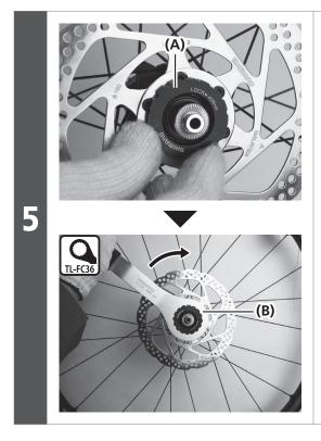
Tighten the disc brake rotor fixing lock ring.
