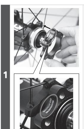
Place the disc brake rotor adapter on to the hub.
