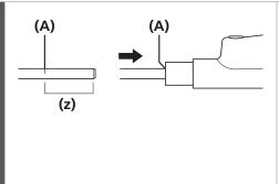
In order to check that the ends of the hose are fitted securely into the base of the hose mounts of the brake calipers and brake lever, make marks on the brake hose beforehand as shown in the illustration.
