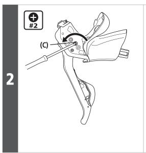
Turn the free stroke adjustment screw to adjust the stroke.
