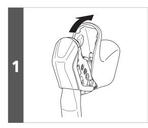
Unhook both the right and left tabs of the bracket cover and open up the bracket cover as shown in the illustration.
