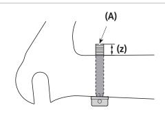
Insert the converter fixing bolts into the frame mount area, and check that the lengths of the protruding sections of the converter fixing bolts are 13 mm.
