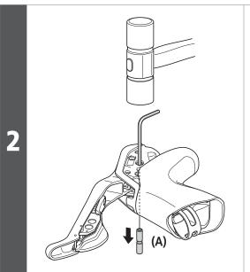
Insert an hexagon wrench or a similar tool into the hole in the lever stud, and then tap it with a plastic mallet to push out the lever stud.
