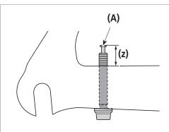
Insert the brake caliper mounting bolts C into the frame mount area, and check that the lengths of the protruding sections of the brake caliper mounting bolts C are 13 mm.
