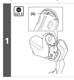
Open up the bracket cover and remove the name plate fixing screw.
