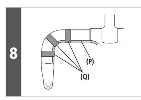
Temporarily secure the brake hose to the handlebar (by using tape or similar material).
