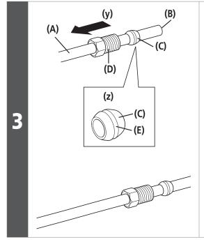
Pass the brake hose through the connecting bolt and olive, as shown in the illustration.
