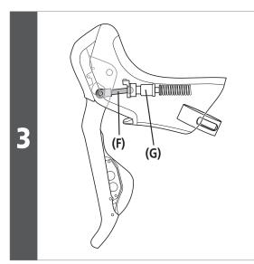
Set the lever unit to the bracket unit in
