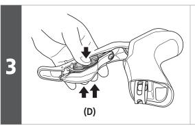
Press the switch unit by hand so that the switch springs go into the grooves in the buttons, and then push the shifting switches (X / Y) in as far as they will go.
