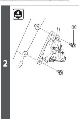
Attach the adapter temporarily to the frame.
