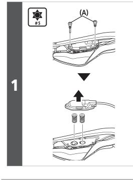
Remove the two switch unit fixing screws, and then remove the switches and the switch springs.
