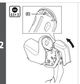
Open up the bracket cover and remove the name plate fixing screw.
