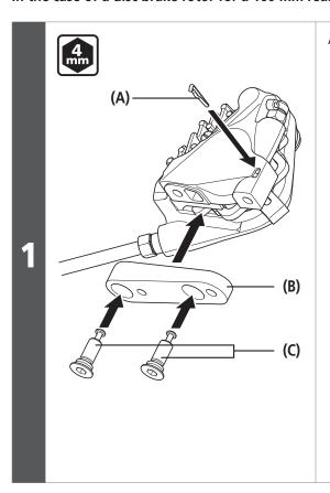
Attach the adapter to the brake caliper.
