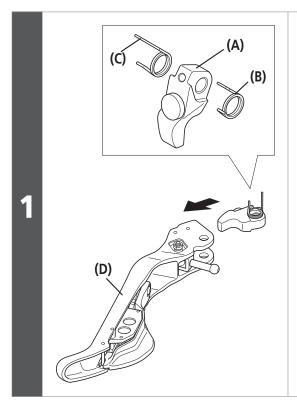
Mount the fixing spring (R) and fixing spring (L) to the cam, and mount the cam to the lever unit.
