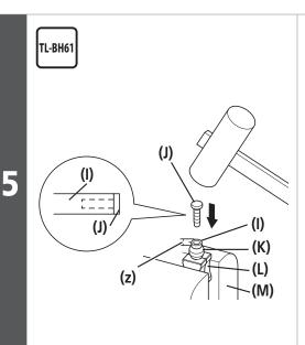
Use a tapered tool to smooth out the inside of the cut end of the brake hose, and mount the connector insert.
