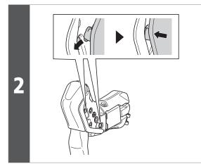
Insert the lower protrusion into the appropriate hole of the bracket unit, and then insert the upper protrusion.
