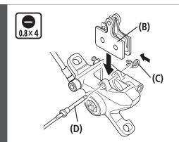
Install the new brake pads and bolts. At this point, make sure to install the snap ring as well.
