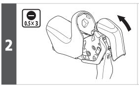
Hold the lower part of the name plate while gripping the lever, and pull up the name plate to remove it as shown in the illustration.
