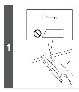
Use a utility knife or other cutting tool to cut the brake hose.
