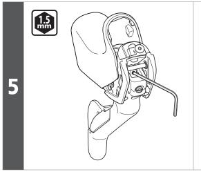
Tighten the lever mounting bolt with an hexagon wrench.
