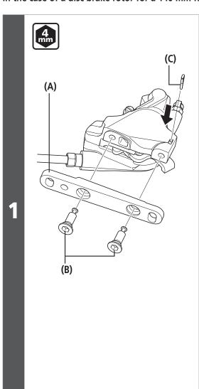
Attach the adapter to the brake caliper.
