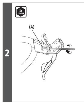
Install the dual control lever to the handlebar and tighten the clamp nut with an hexagon wrench.
