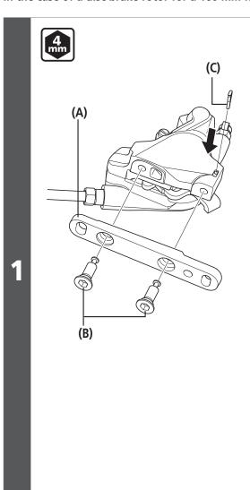
Attach the adapter to the brake caliper.
