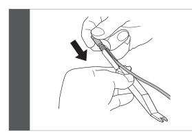
Set so that the projection on the connector is aligned with the groove on the narrow end.
