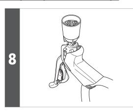
Once there are no more air bubbles in the oil in the funnel, temporarily close the bleed nipple / screw.
