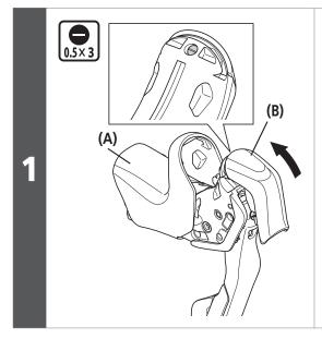
Open up the bracket cover and remove the name plate.
