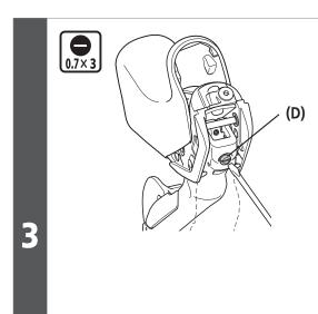
Turn the reach adjustment screw to position the lever unit.
