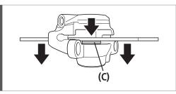
Use a flat-shaped tool to push the pistons straight back in as far as they will go, while being careful not to twist the pistons.
