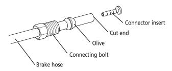
• Cut the brake hose so that the cut end is perpendicular to the length of the hose. If the brake hose is cut at an angle, fluid leaks may result.
