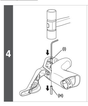
Use an hexagon wrench to install the lever stud.
