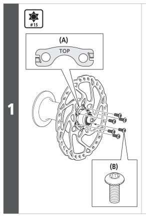
Install the disc brake rotor and rotor lock washers to the hub and tighten the bolts.
