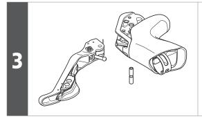
Remove the lever unit from the bracket ..
