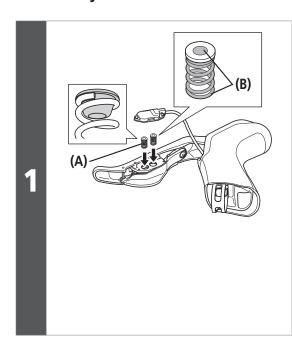
Check that the buttons are attached to the springs, and then place the switch springs into the holes in the switch unit setting plate.
