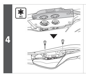
Make a gap between the switch unit and the switch unit setting plate and check that the end of the rubber on the switch unit is on the button.
