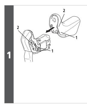
Insert the protrusions of the bracket cover as shown in the illustration.
