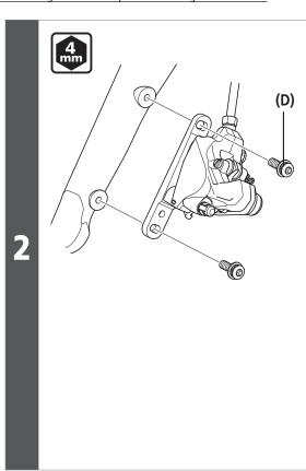
Attach the adapter temporarily to the frame.
