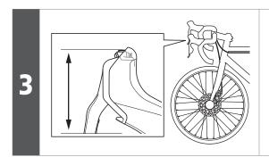
Adjust the position of the bleed screw so that its surface is parallel to the ground.
