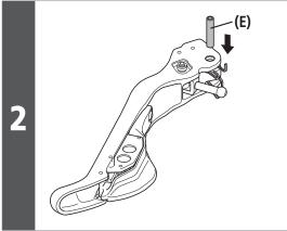
Temporarily assemble the cam and lever unit by TL-ST04.
