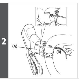
Use the TL-EW02 to connect the connector of the electric wire to the terminal on the lever side.
