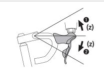
Tilt the handlebar in the up/down directions by 30 degrees as shown in the illustration, and then perform step 13 to check that there is no air bubble remaining.
