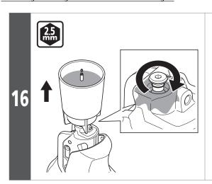
Remove the oil funnel while it is still being plugged with the oil stopper, and then attach the O-ring to the bleed screw and tighten it while letting oil flow out to make sure that there are no air bubbles remaining inside the reservoir tank.
