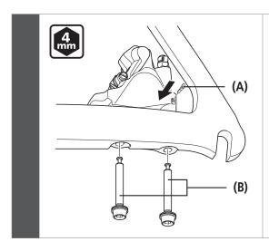
Attach the brake caliper to the frame.
